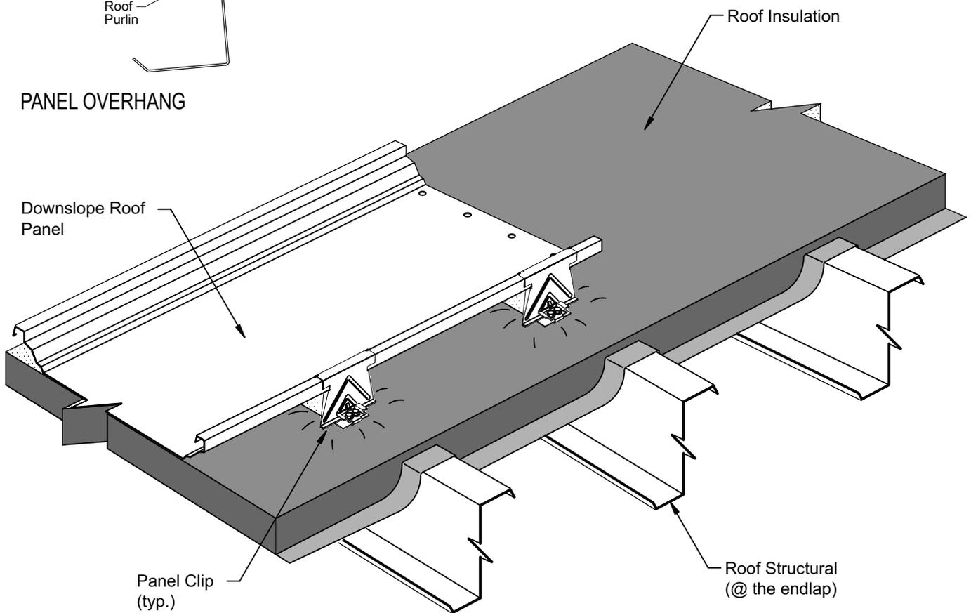
With the eave end of the roof panel attached, measure the panel overhang at the purlin (see illustration).
