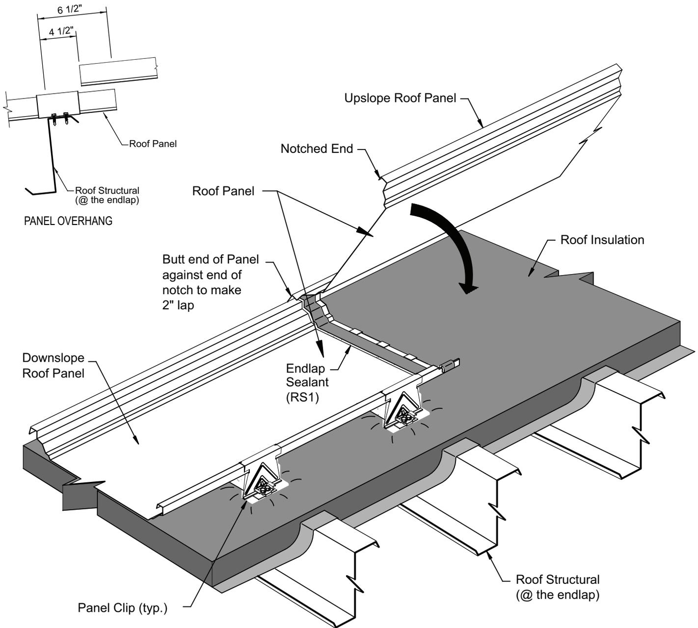
Wipe dry and clean the underside surface of the up-slope roof panel.
