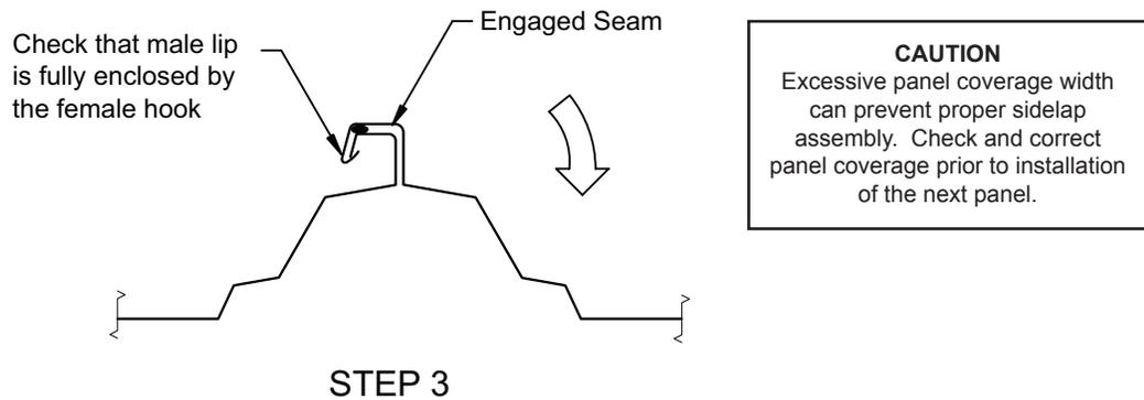
It is easier to hook the roof panel seams together if the roof panel is first tilted up to the vertical position.
