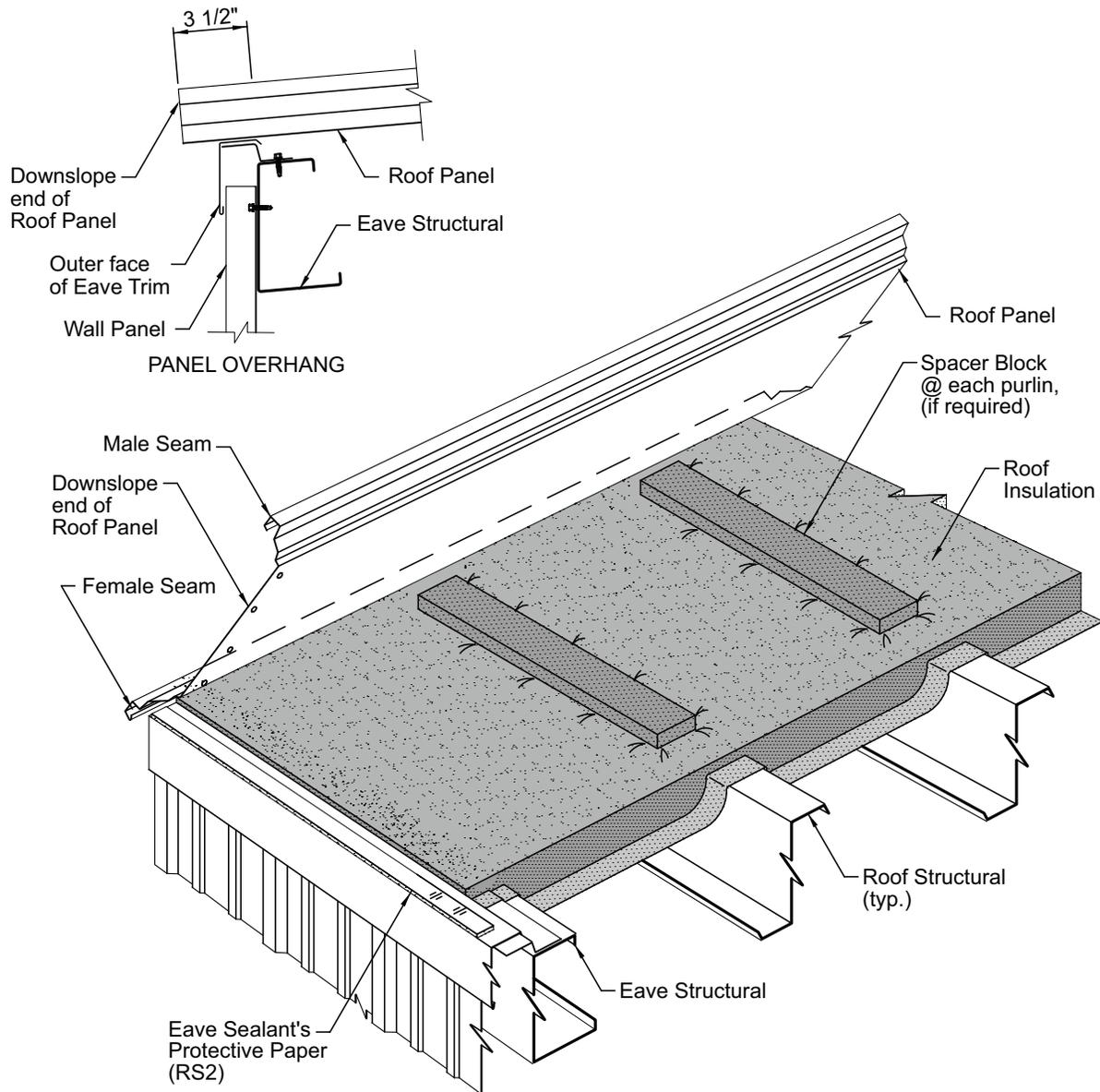
The roof panel's eave overhang dimension is critical as it establishes the location of endlaps and ridge cover attachment points.
