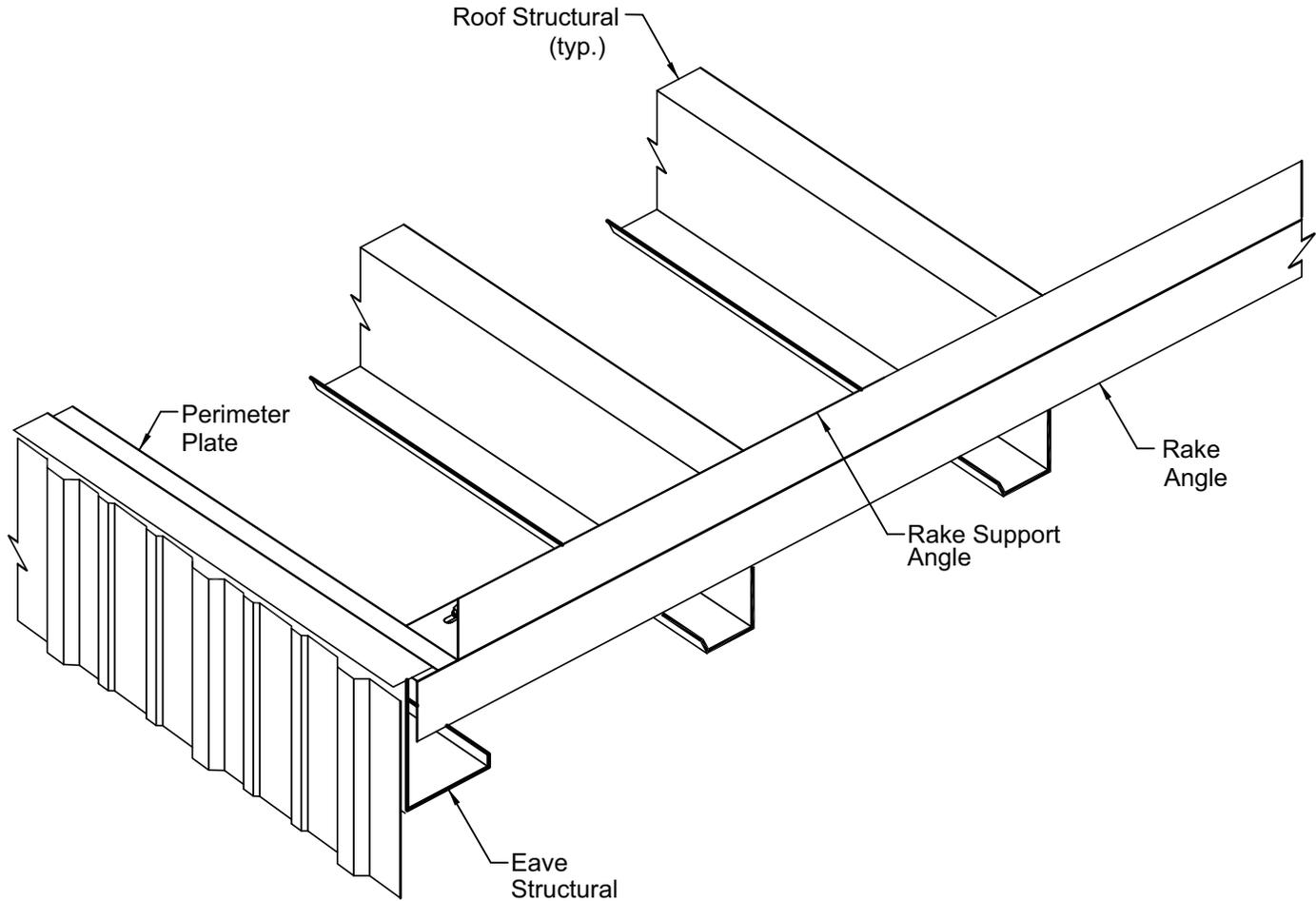
It is important that the rake support angle is installed in a straight line and parallel to the rake line.
