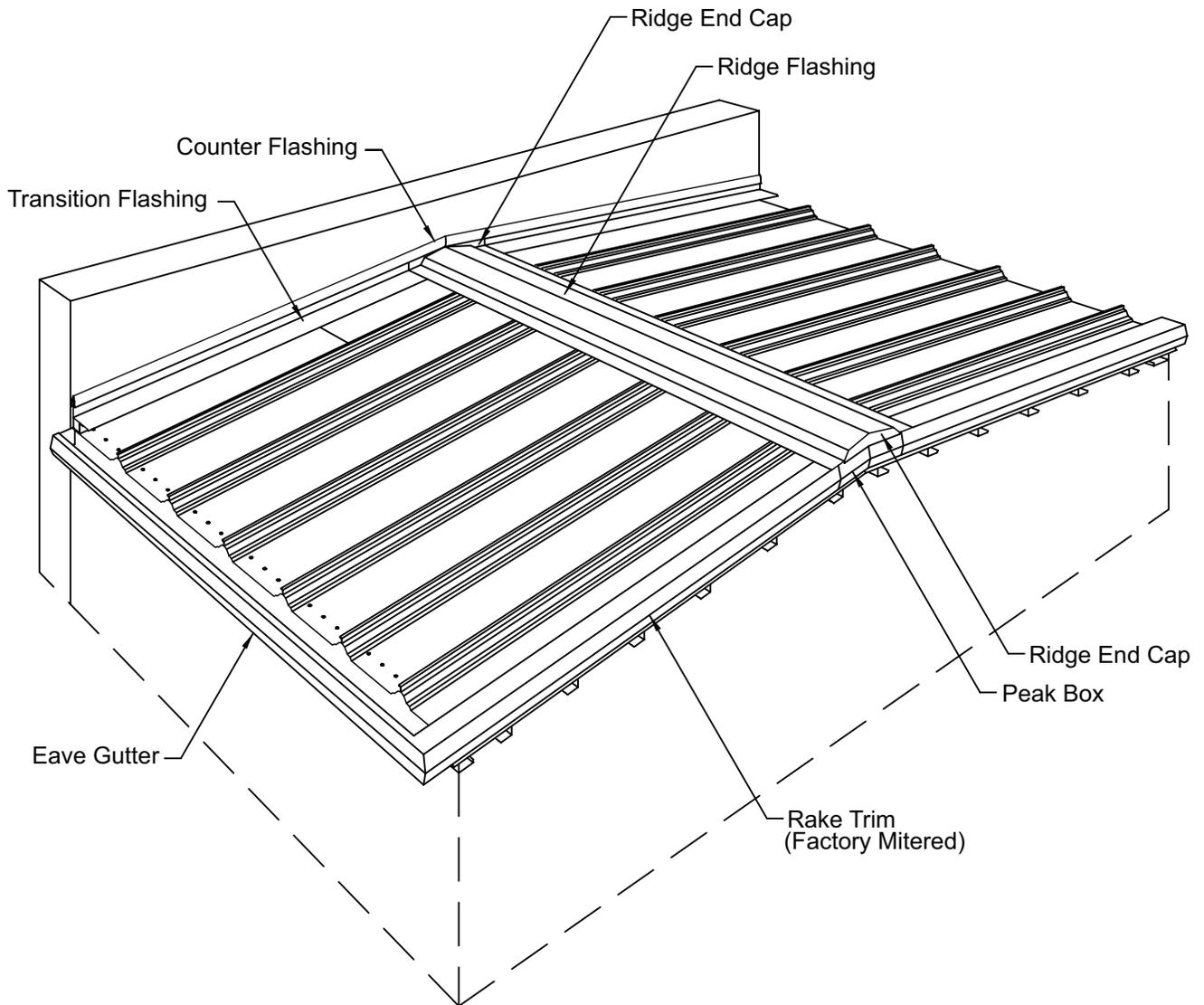
The details in this section show assembly and installation of eave gutter.
