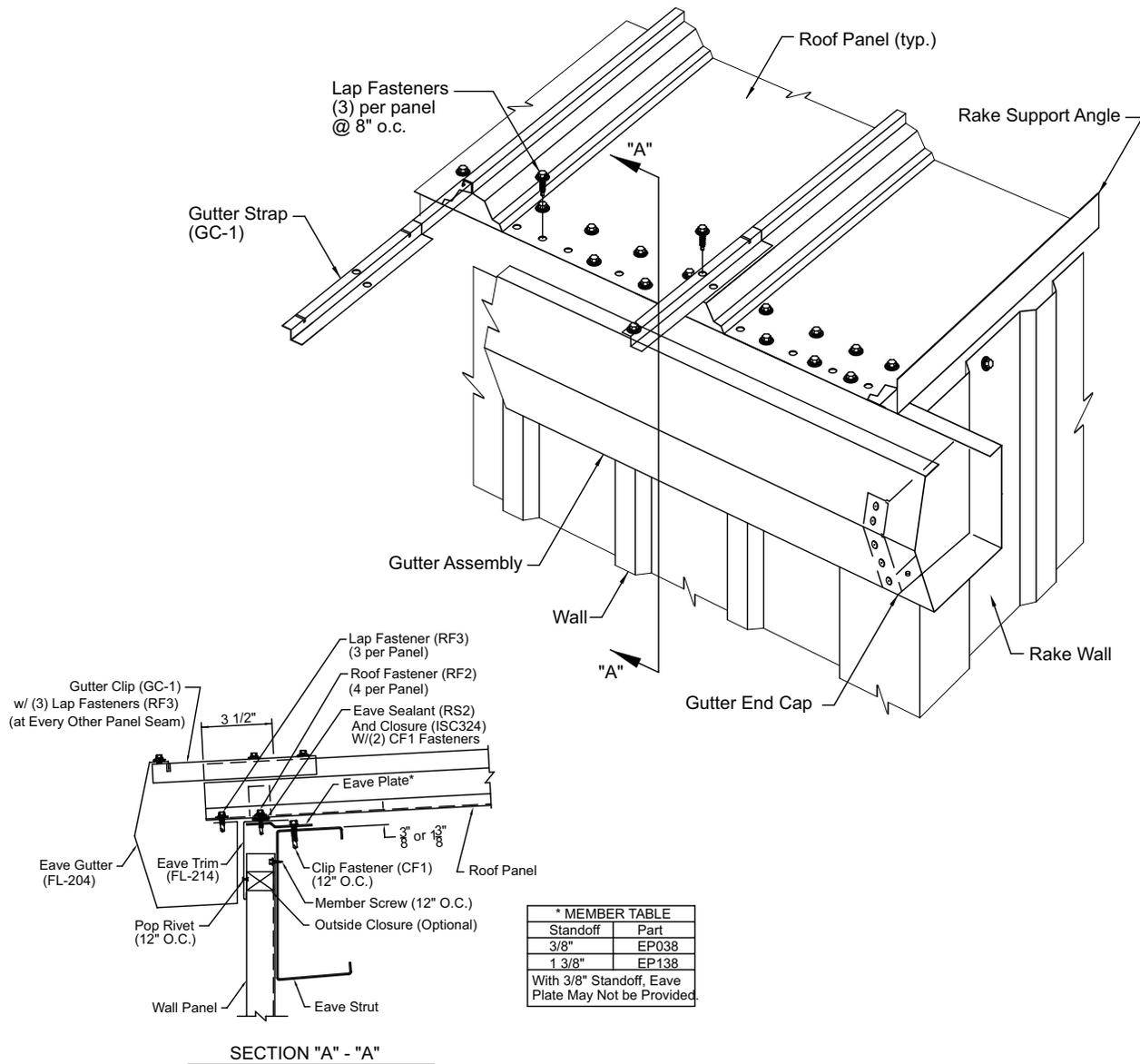
Lift the gutter assembly into position under the edge of the roof panels and temporarily clamp the back flange of the gutter to the roof panel.
