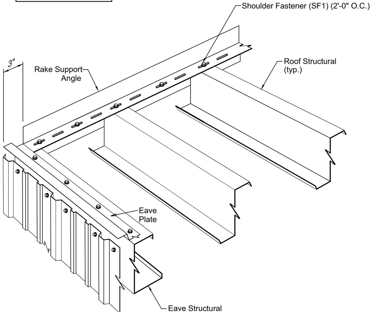
The appropriate height rake support angle is used.
