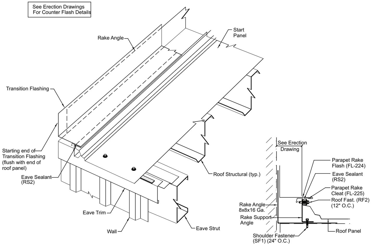
Install the transition flashing from eave to ridge to provide for watershed at the splices.
