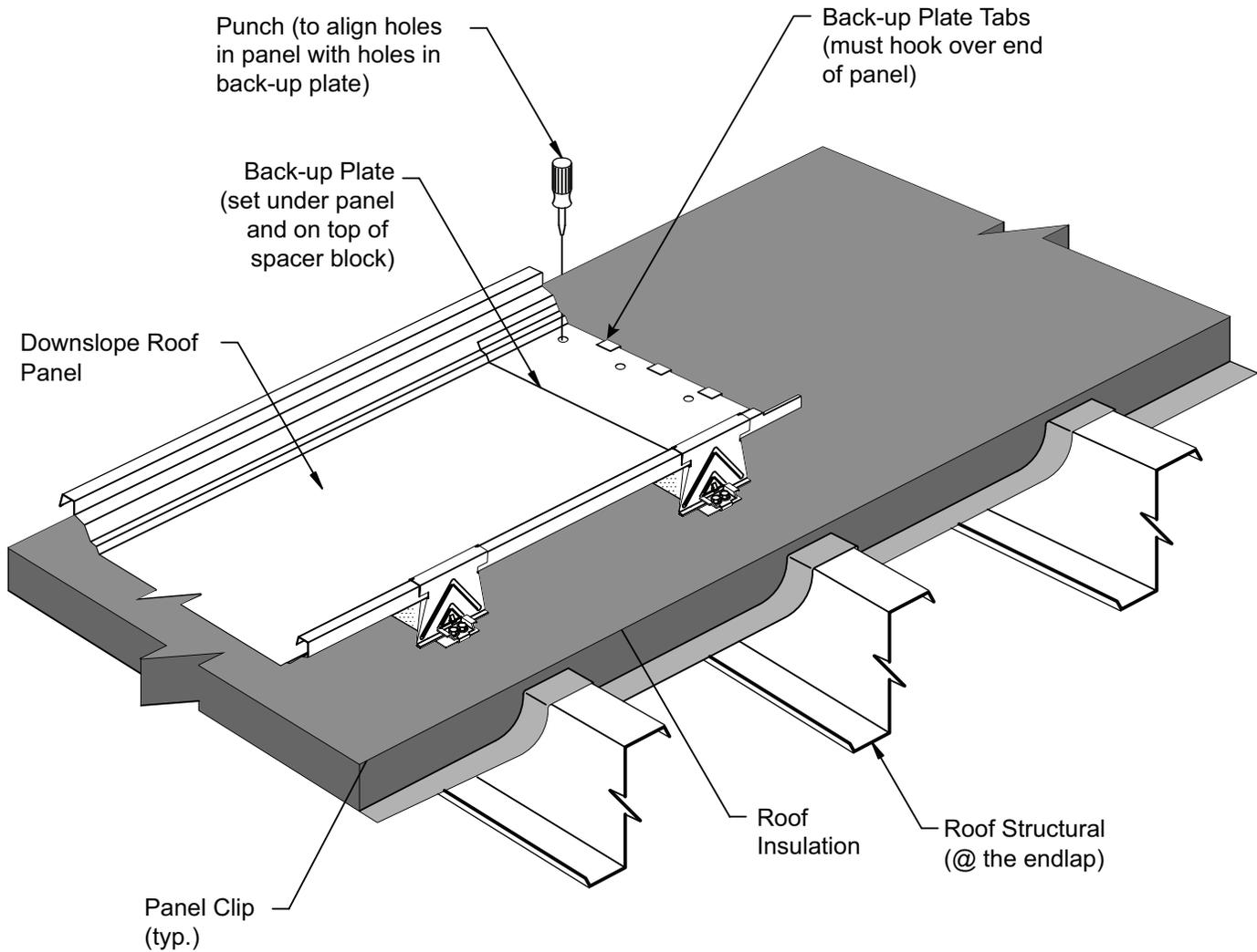
NOTE: Leading edge of back-up plate must be trimmed at rake to allow panel high rib to sit flush against rake support angle
