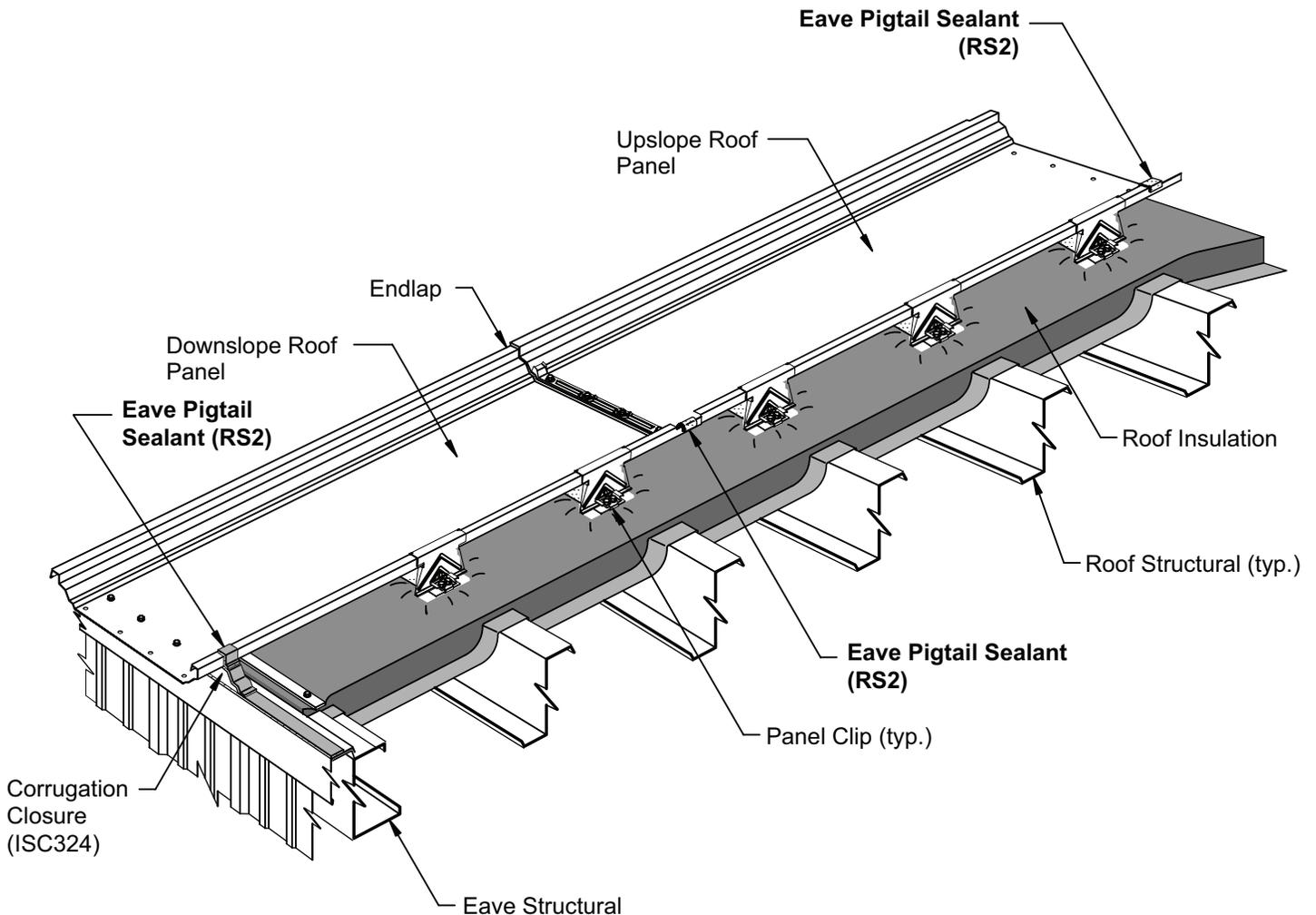
**The eave pigtail sealants must be correctly installed before** the next roof panel run can be installed.
