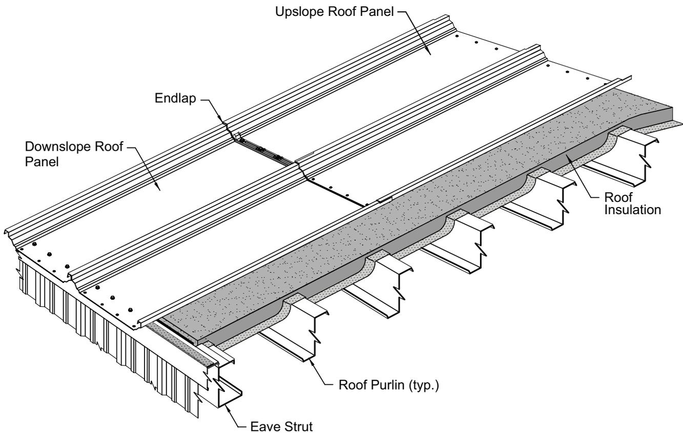
The most common coverage error is the spreading of the roof panels, especially at the panel ends. This can cause excess panel coverage along the eave, endlaps and ridge.
