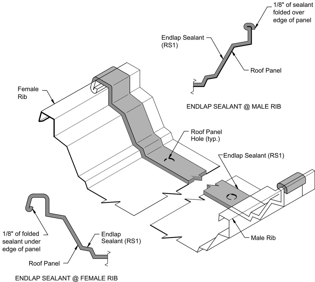
Cut the endlap sealant to be fitted around the roof panel's seams as shown.
