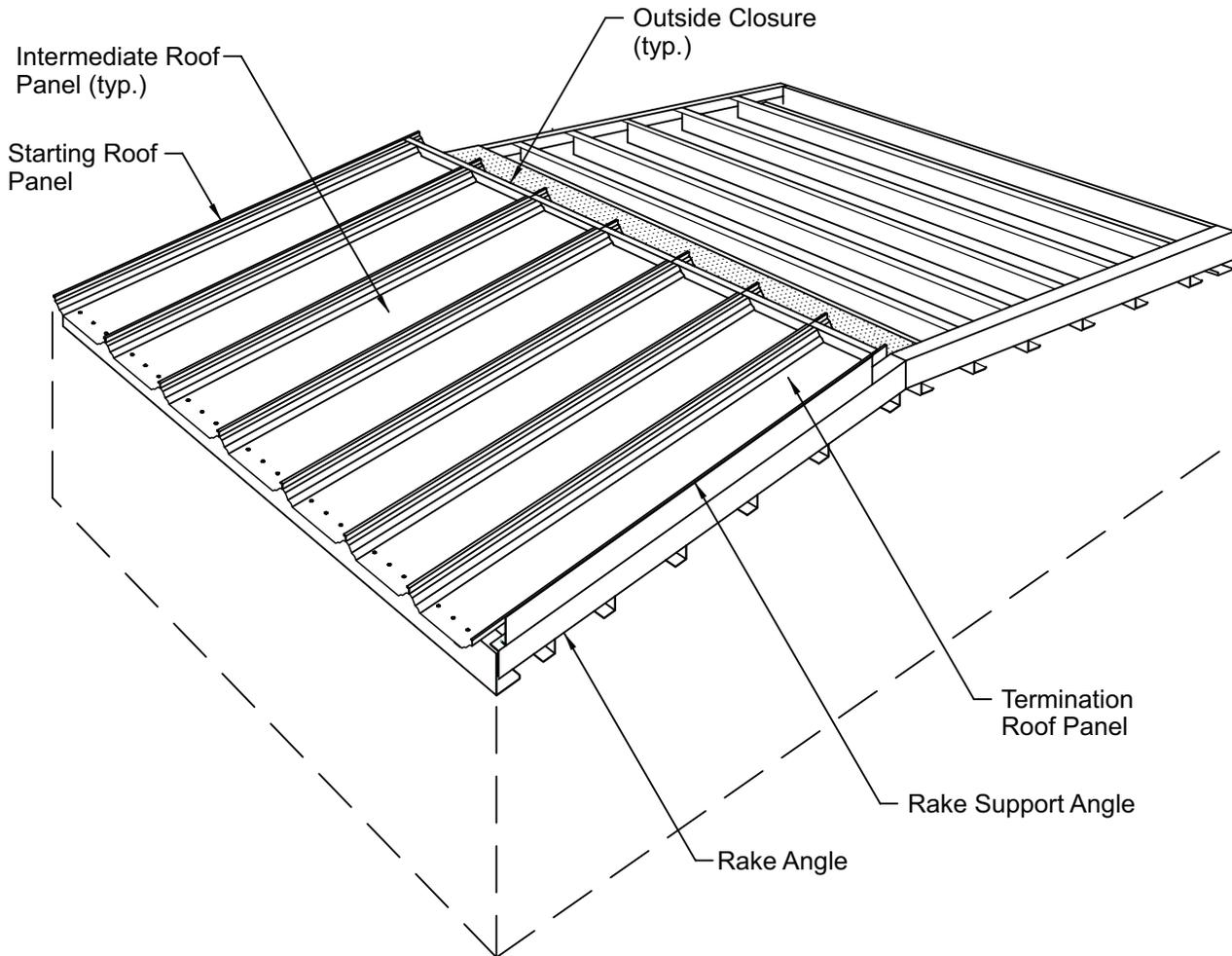
Metal outside closures are used to close the ends of the roof panels at the ridge, high eave and high eave transition conditions.
