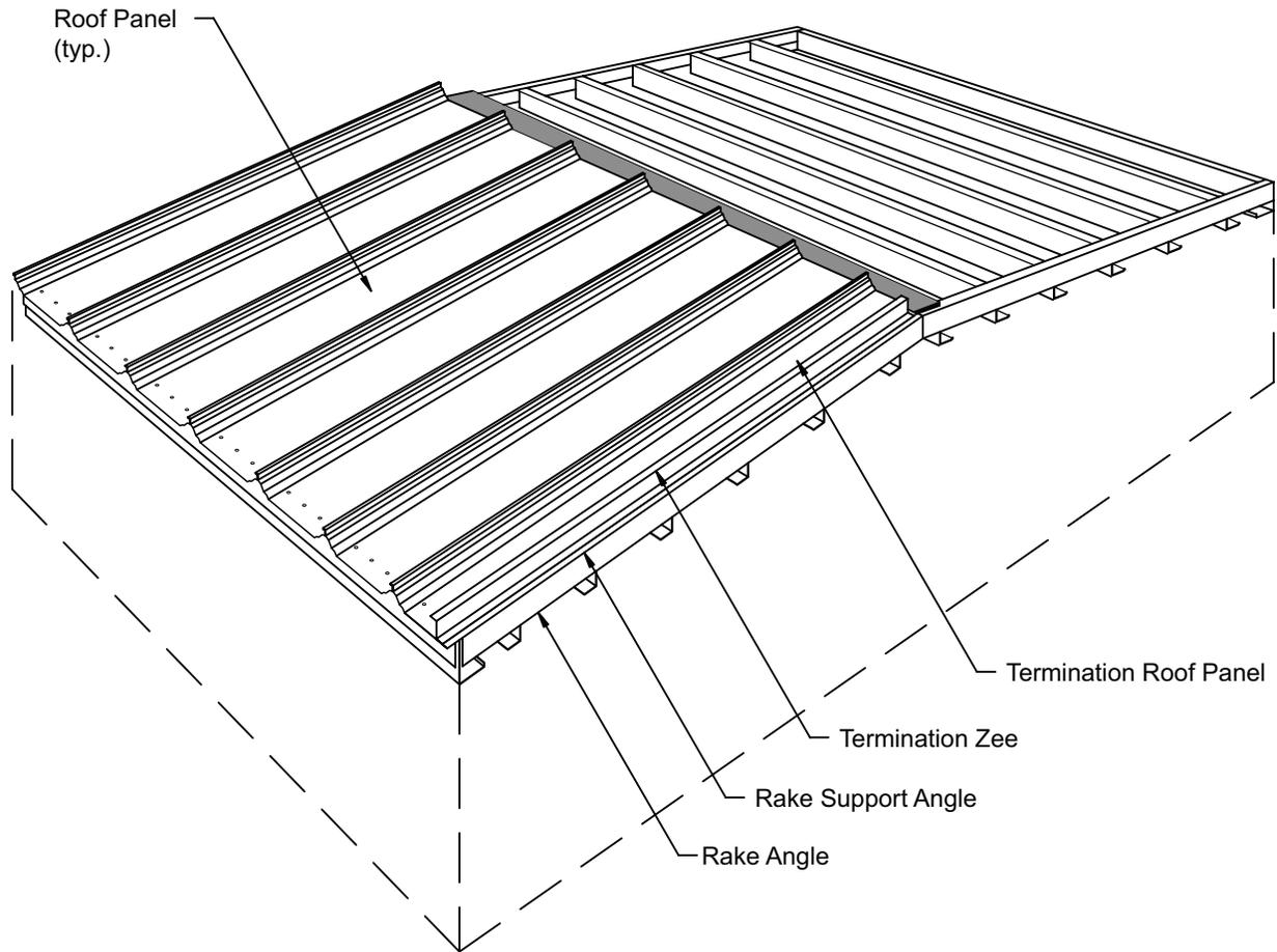
The details in this section show the installation of the termination roof panel.
