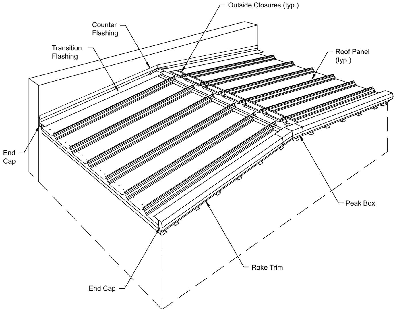
Note: Parapets or existing buildings should extend 1'-0" minimum above roof panels.
