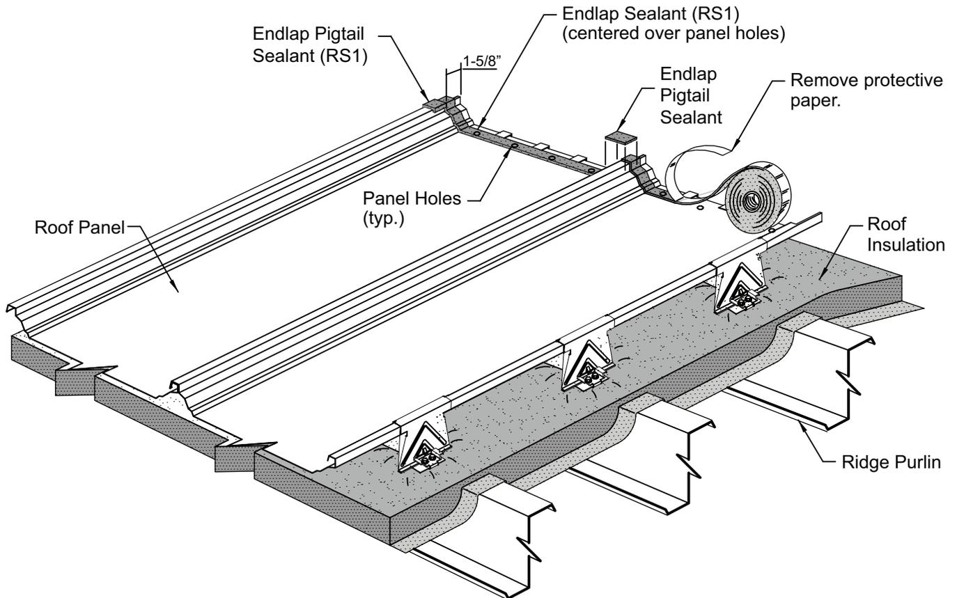
Before installing the endlap sealant, the roof panel's surface must be wiped clean and dry.
