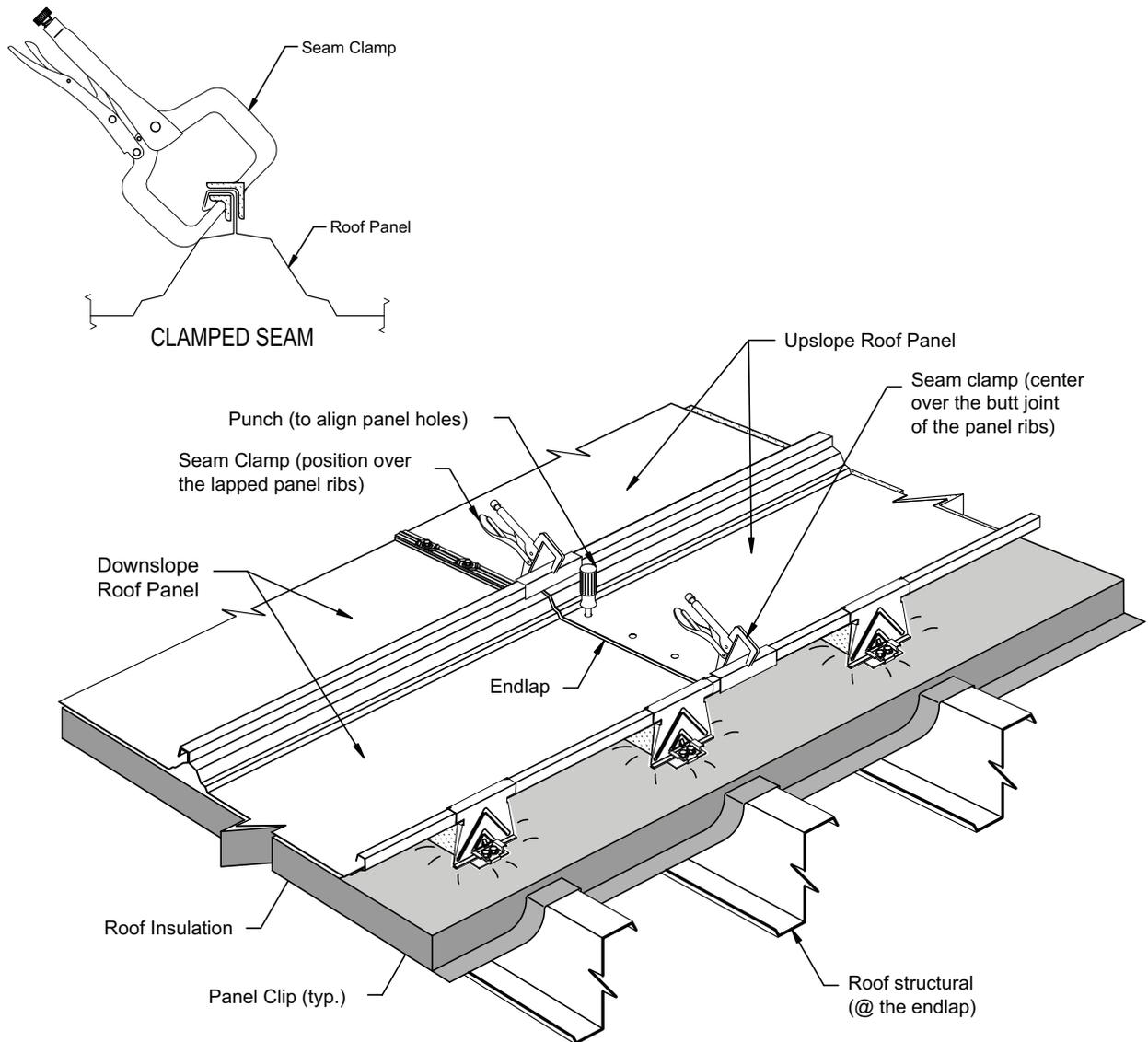
Use the seam clamps to draw the lapping panel seams together, as shown.
