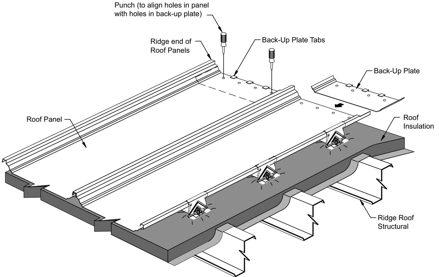
Slide the back-up plate under the roof panel as shown.
