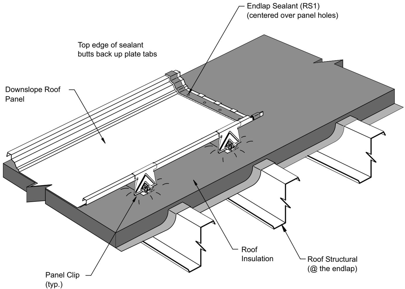
The proper placing of the endlap sealant is critical to the weather tightness of the roof endlaps.
