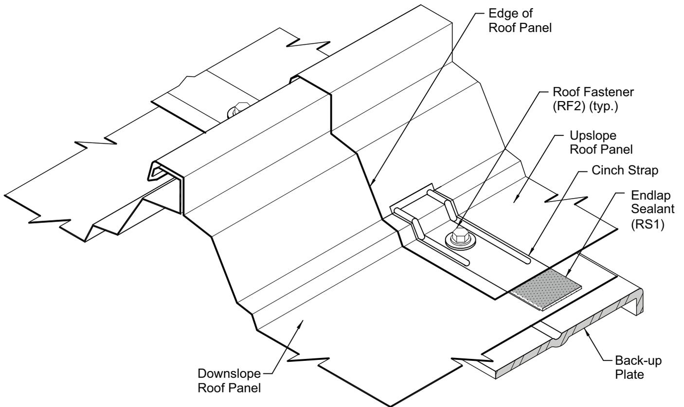
Check that the endlap is correctly assembled as shown.
