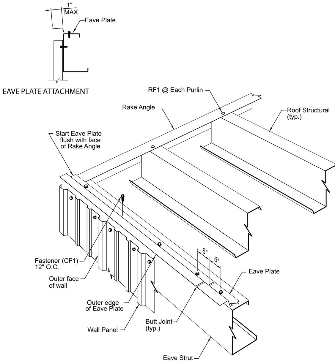
The eave plate may or may not be required when the first purlin space is greater than 4'-0". See erection drawings to determine if eave plate is required.
