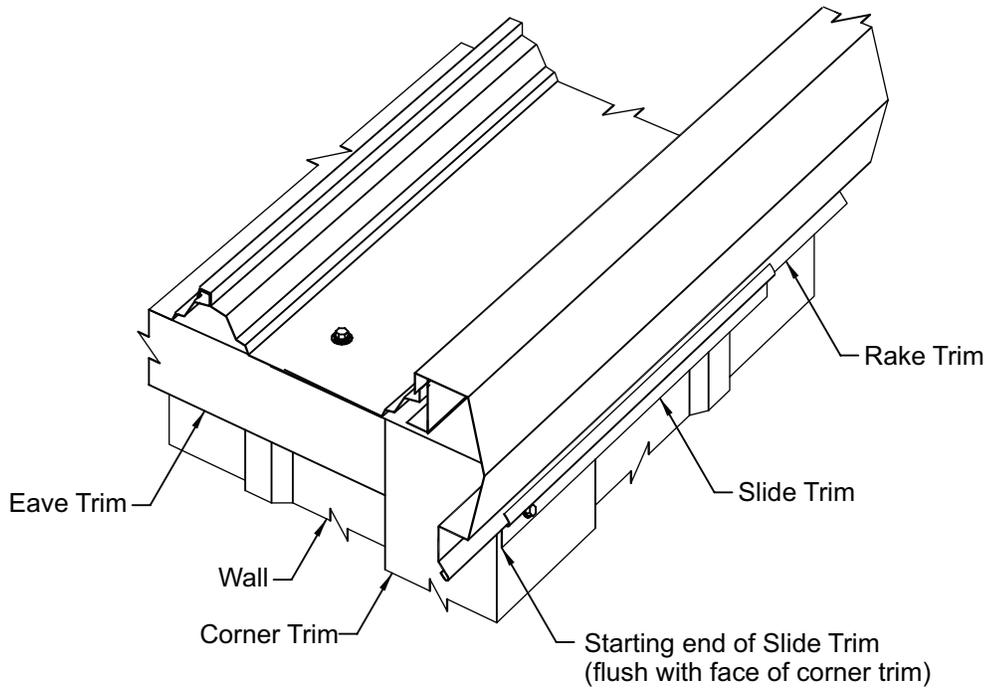
The bottom edge of the rake trim must be secured with the slide trim to allow for roof expansion/contraction.
