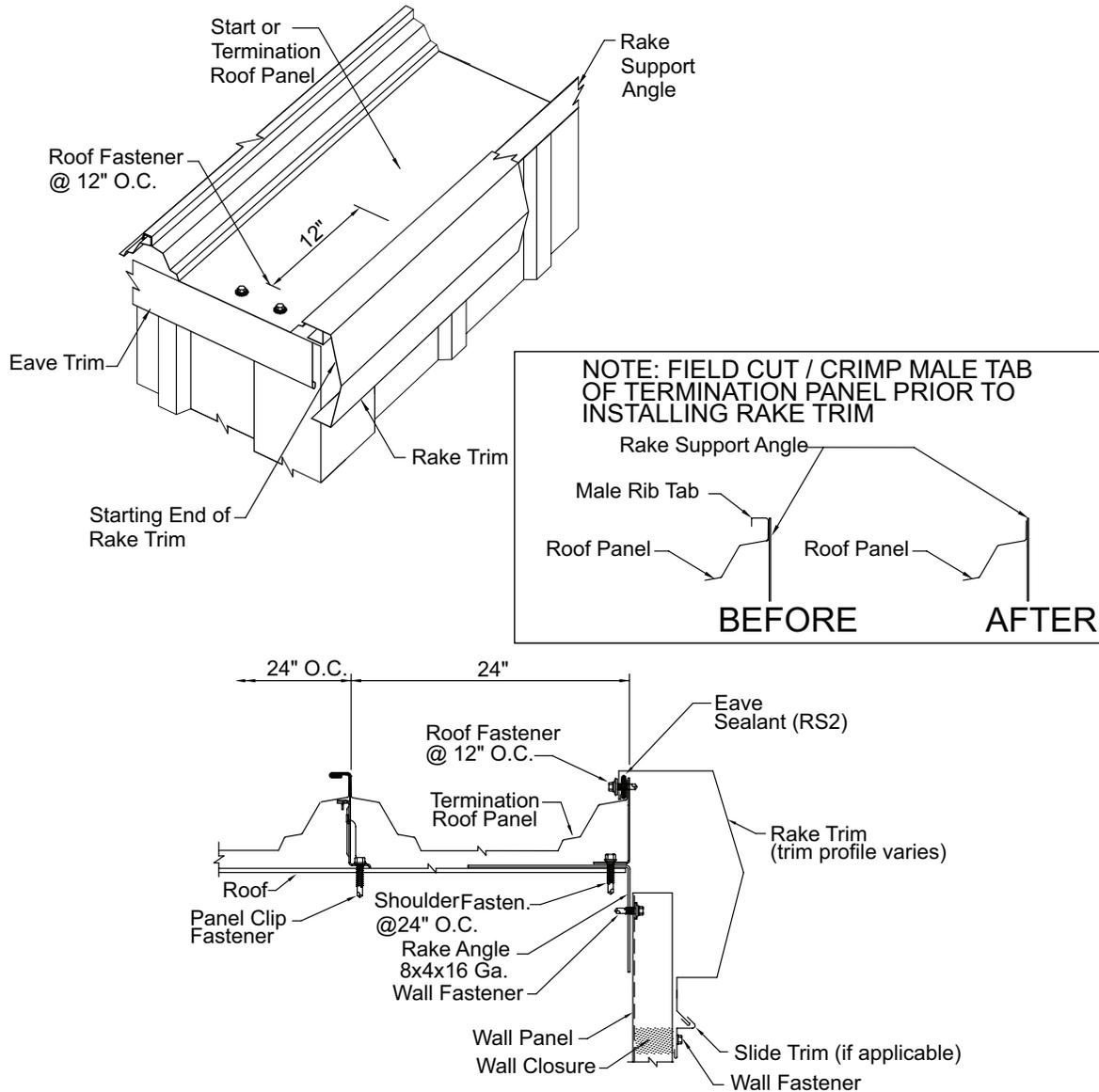
Install the rake trim from eave to ridge to provide for watershed at the splices.
