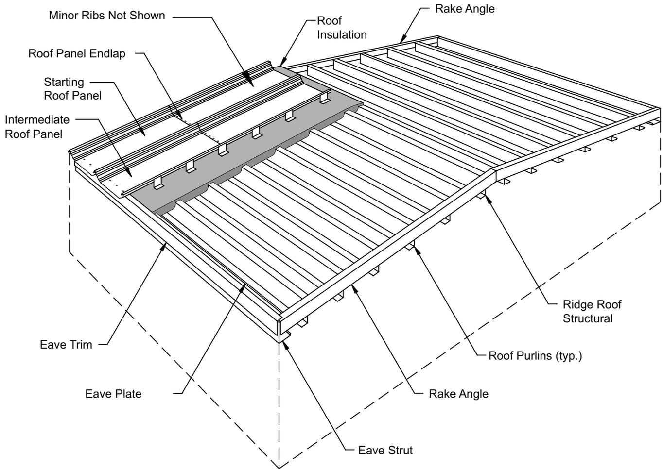
The details in this section show the installation of the starting and intermediate roof panels.
