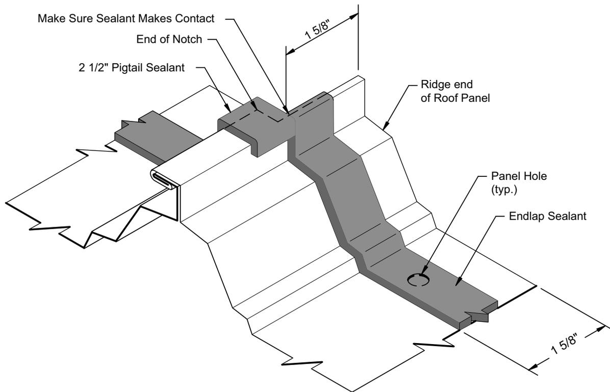
The correct installation of the ridge sealant is critical to the weather resistance of the roof system.
