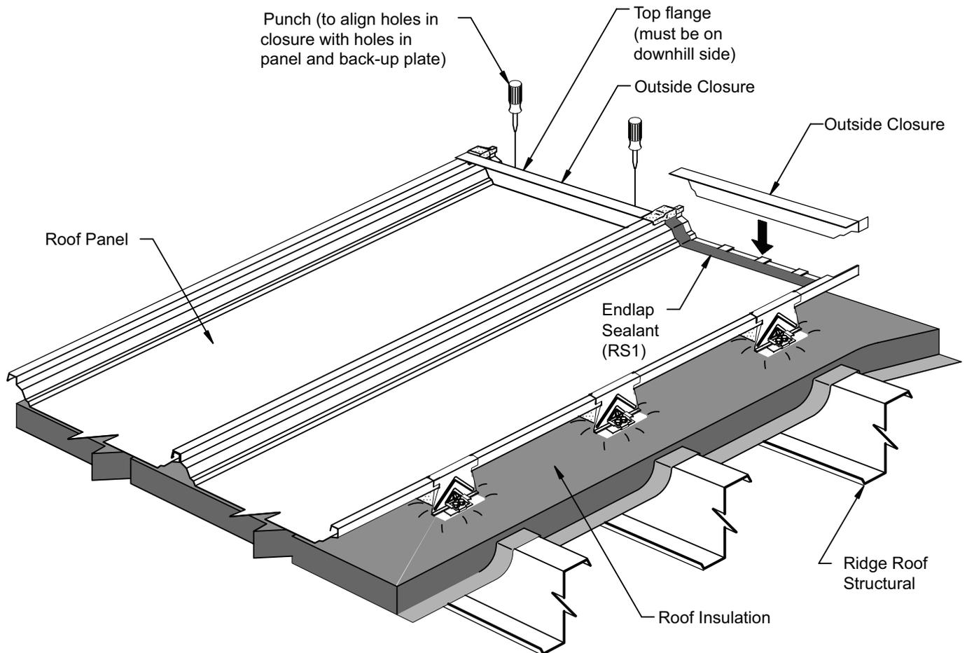
Wipe dry and clean the underside surface of the outside closure flanges.
