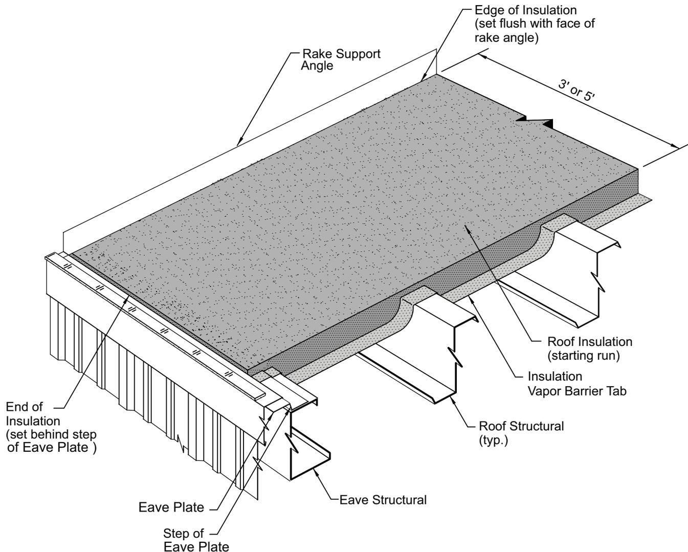
Refer to the purchase order to determine the specific insulation required for the project. In all cases refer to the insulation manufacturer's instructions for proper insulation installation and vapor seal assembly. This detail shows fiberglass blanket insulation, which is the most commonly used insulation for metal standing seam roofs.
