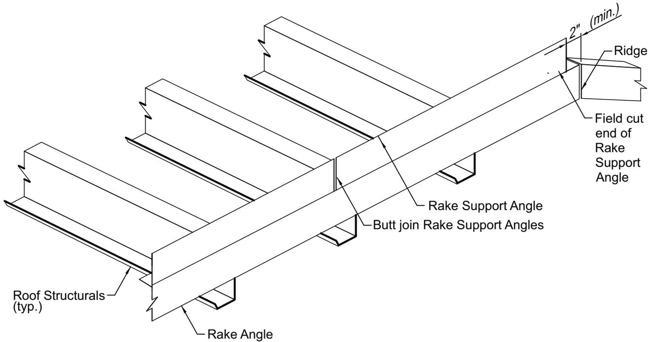
Butt join the ends of the rake support angle. Install the shoulder fasteners in the slots on either side of the butt joints.
