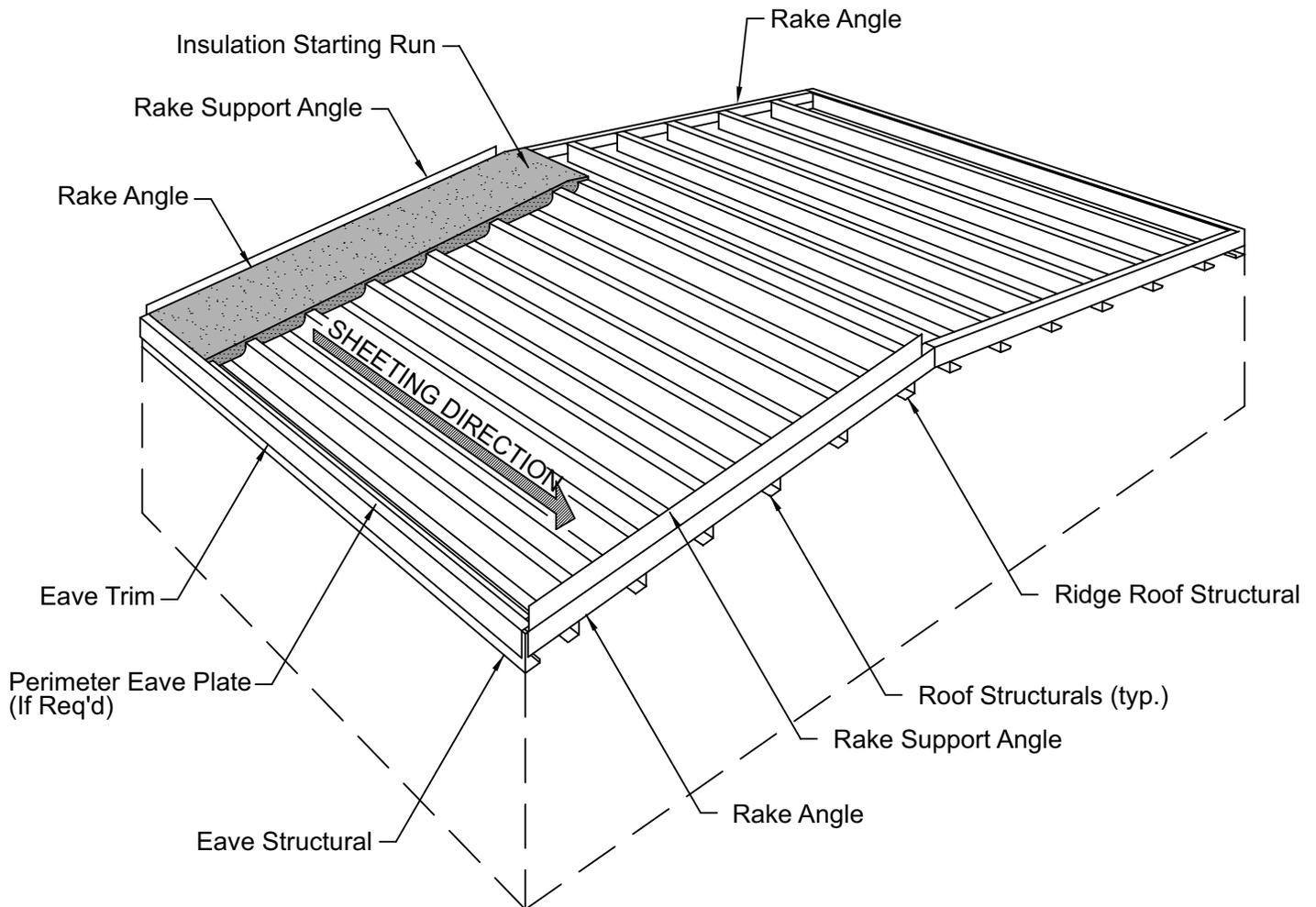
The details in this section will show the installation of the eave plate (if req'd), rake support angle, trim, sealant and the first run of insulation. These are parts that must be installed before the roof panel installation can begin.
