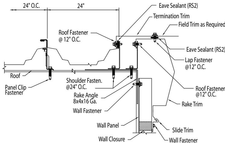
Install the rake trim from eave to ridge to provide for watershed at the splices.
