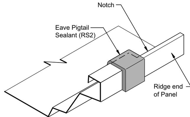
EAVE PIGTAIL SEALANT DETAIL
