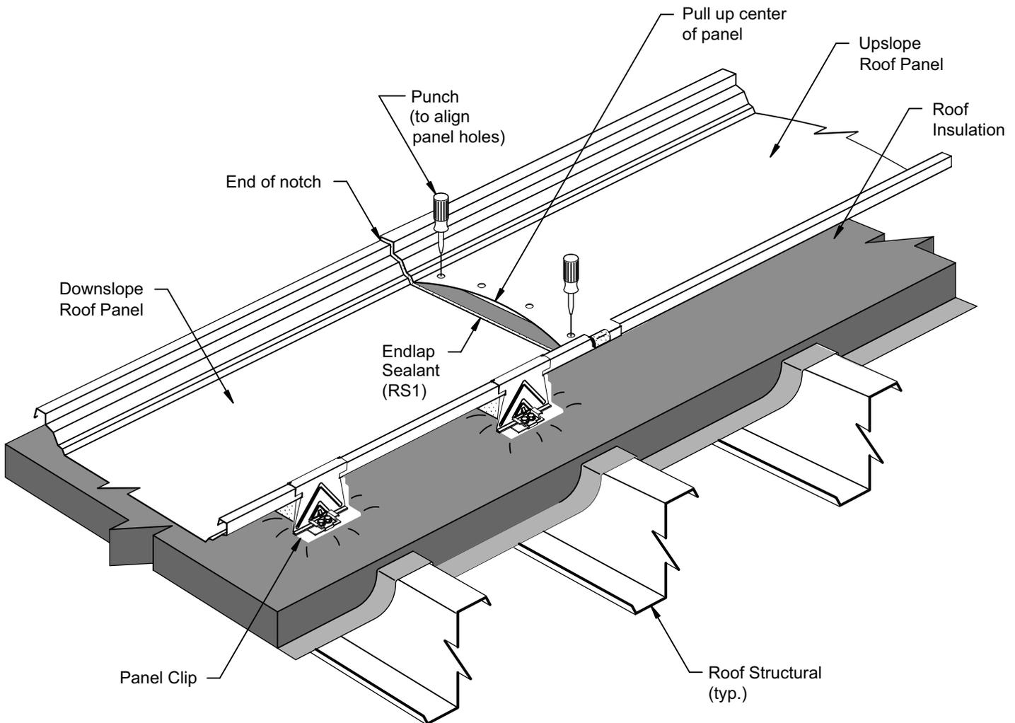
Lower the up-slope roof panel to lap onto the down-slope roof panel.
