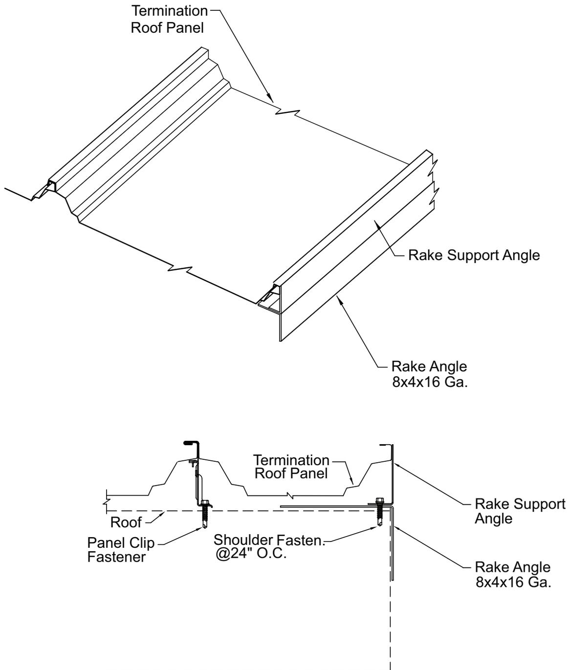
If termination roof panel ends on module at finishing rake, male seam of panel should be against rake support angle.
