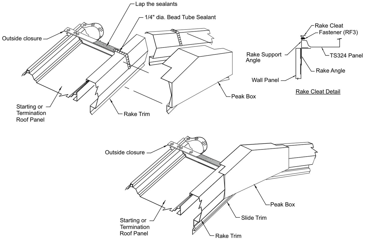
Install rake cleat as shown between rake support angle and peak.
