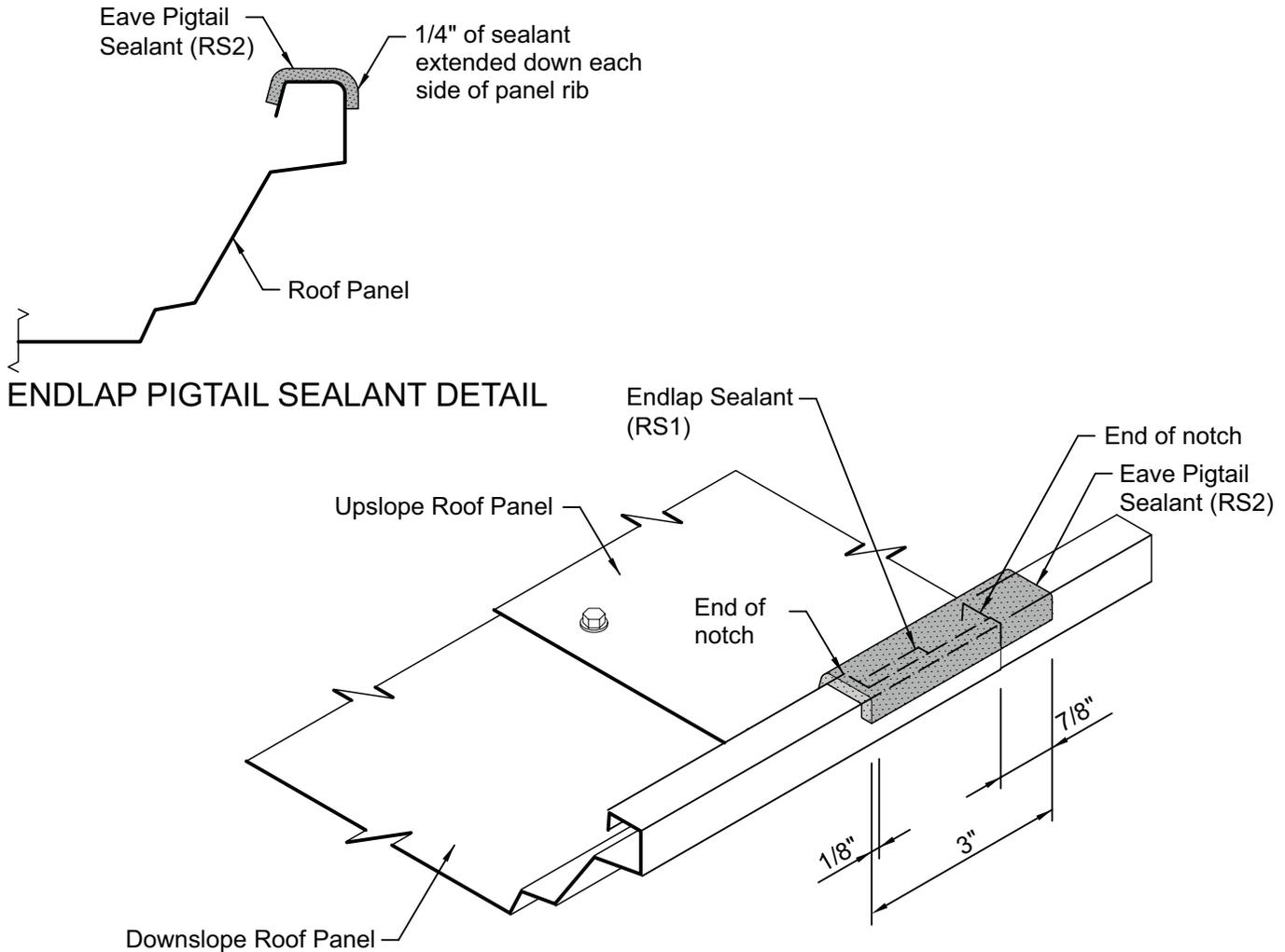
Cut the pigtail sealant to a 3" length and fit around the roof panel's seam as shown.
