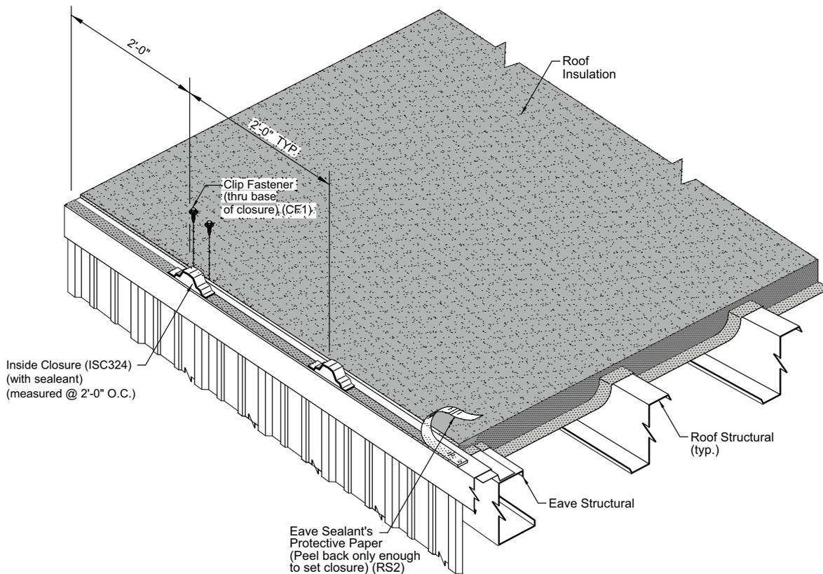
Prepare the corrugation closures by applying eave sealant along the top surfaces as shown in the above illustration. Remove the protective paper.
