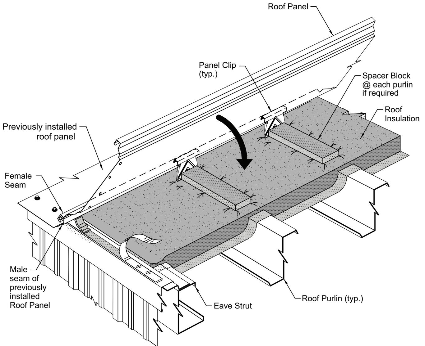
Repeat previous steps of first panel run and remove the protective paper from the eave sealant. Remove only enough of the protective paper to allow installation of the next roof panel.
