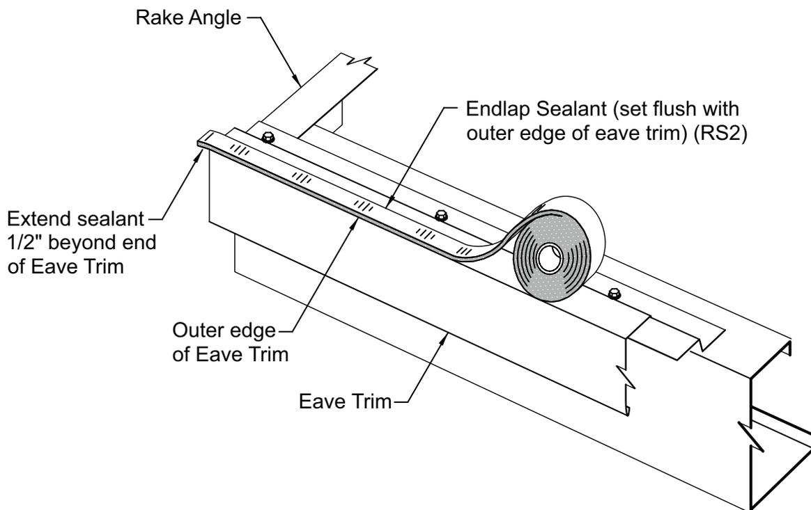
Apply a continuous strip of endlap sealant along the top edge of the eave trim.
