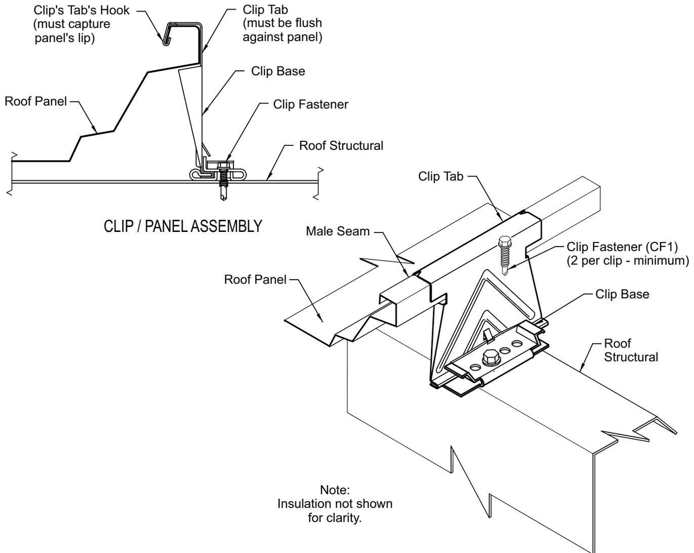
Panel clips are available as floating clips or fixed clips and are available in different stand-off heights. Refer to the erection drawings to determine the type of clip required for each roof condition.
