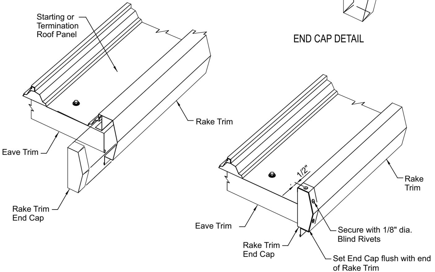
The rake trim end cap is only required for roof applications without eave gutter.
