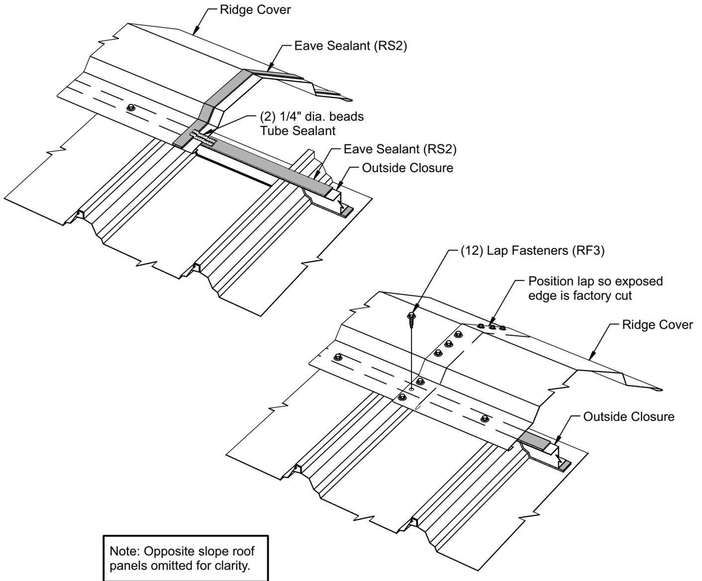
Assemble the ridge cover splices with eave sealant and lap fasteners as shown.
