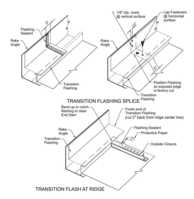
Assemble transition flashing splices with flashing sealant and lap fasteners as shown. Wipe dry and clean the lapping surfaces of the flashing.
