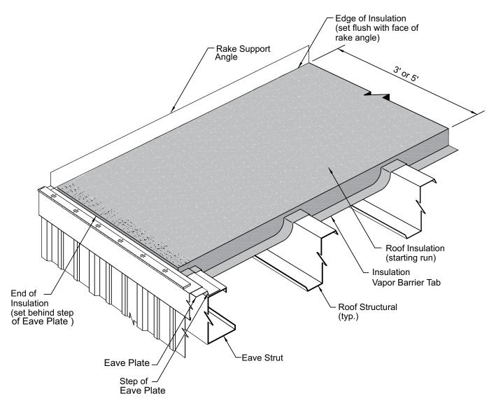
Refer to the erection drawings to determine the specific insulation required for the project. In all cases refer to the insulation manufacturer's instructions for proper insulation installation and vapor seal assembly. This detail shows fiberglass blanket insulation, which is the most commonly used insulation for metal standing seam roofs.
