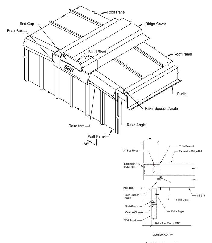
Wall Panel Thickness, Plus Rake Trim Projection, Plus 1/16"
