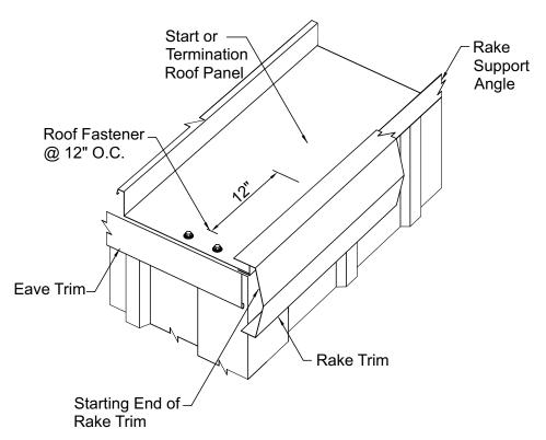
If the roof system is "fixed", the bottom edge of the rake trim can be attached directly to the wall with wall fasteners as shown.
