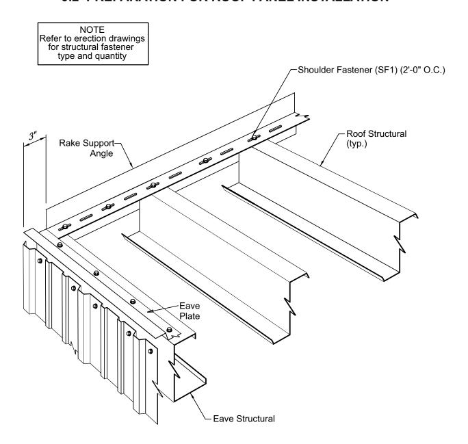
The appropriate height rake support angle is used.
