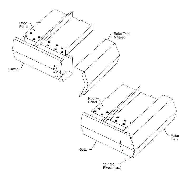
Check to make sure all edges are sealed with tube sealant. Insert the rake trim into the gutter. Align the mitered edges and attach with 1/8" pop rivets.
