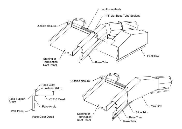
Install rake cleat as shown between outside closure and peak.
