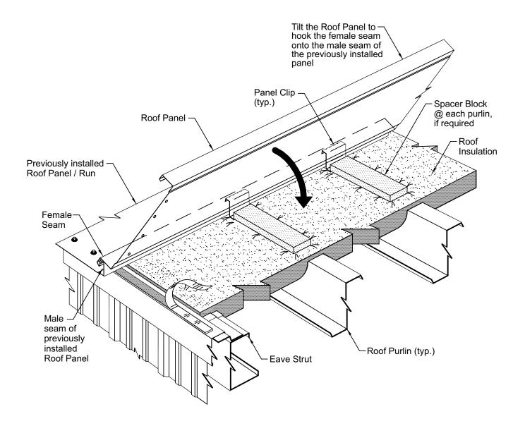
Remove the protective paper from the eave sealant. Remove only enough of the protective paper to allow installation of the next roof panel.
