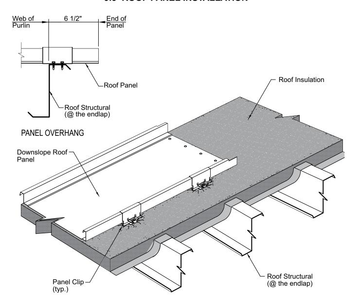
With the eave end of the roof panel attached, measure the panel overhang at the endlap roof structural (see illustration).
