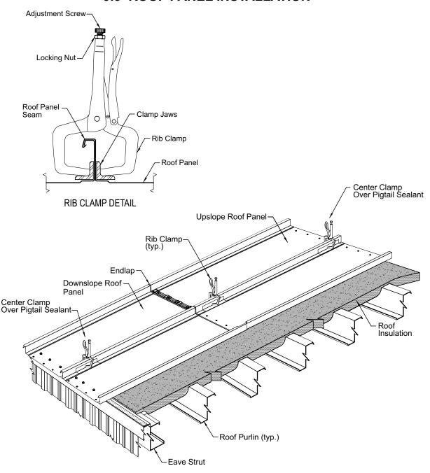
The most common coverage error is the spreading of the roof panel sidelaps, especially at the panel ends. This can cause excess panel coverage along the eave, endlaps and ridge.
