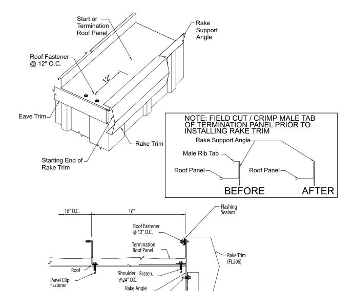
Install the rake trim from eave to ridge to provide for watershed at the splices.
