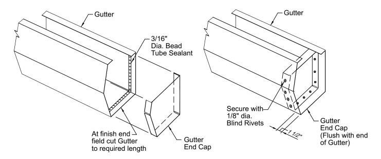
Layout the gutter assemblies before installation on the roof.
