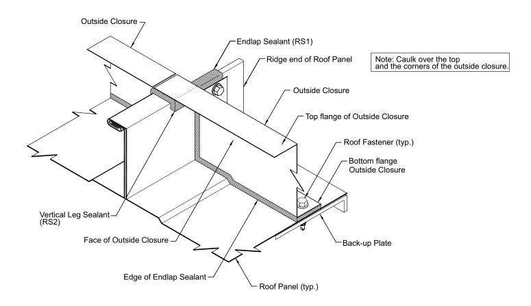
Verify that the outside closure is correctly assembled as shown.
