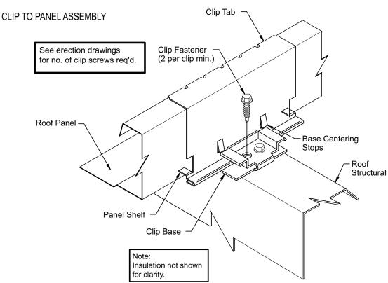
Panel clips are available as floating clips or fixed clips and are available in different stand-off heights. Refer to the erection drawings to determine the type of clip and quantity of fasteners required for each roof condition.
