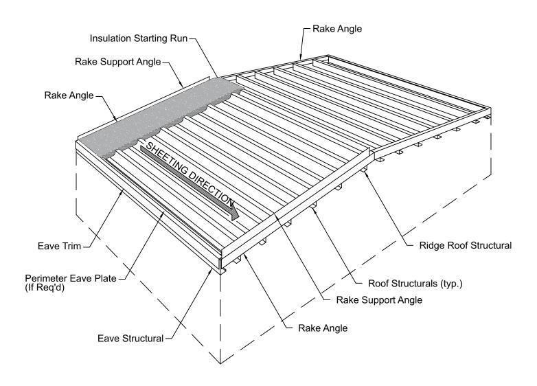
The details in this section will show installation of the eave plate (if req'd), rake support angle, trim, sealant and the first run of insulation. These are parts that must be installed before the roof panel installation can begin.
