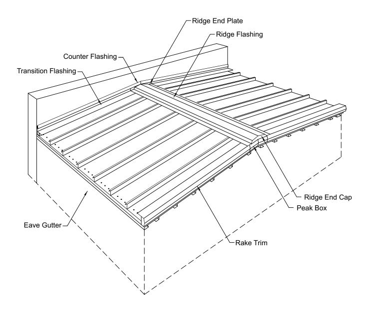
The details in this section show the installation of the ridge cover.
