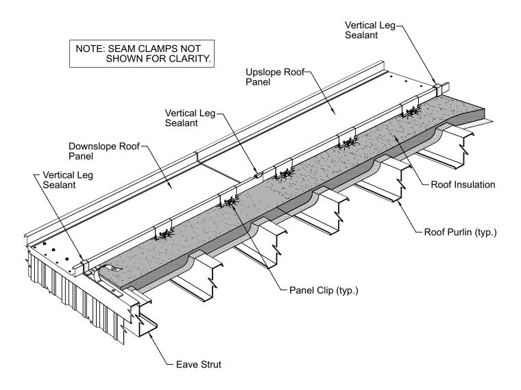
The vertical leg sealants must be correctly installed Refer to the next pages for specific pigtail sealant details. **before** the next roof panel run can be installed.
