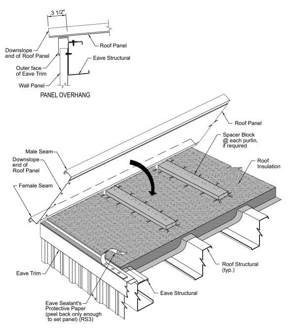
The roof panel's eave overhang dimension is critical as it establishes the location of endlaps and ridge cover attachment points.
