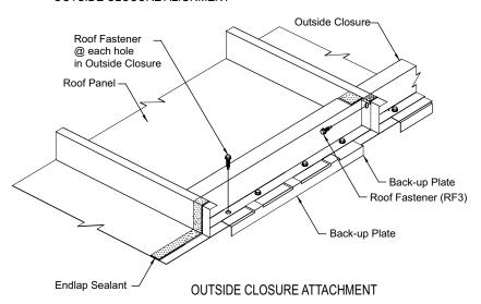
Uniformly press the outside closure into the ridge sealant to assure adhesion. Use a clamp to hold the assembly together while installing the fasteners.
