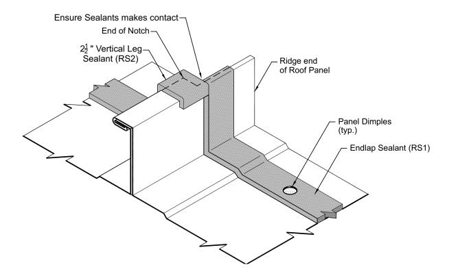
The correct installation of the ridge sealant is critical to the weather resistance of the roof system.
