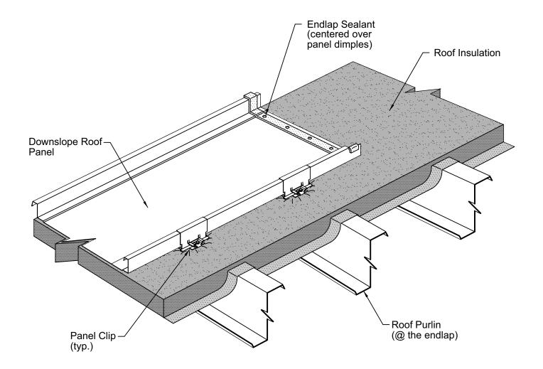
The proper placing of the endlap sealant is critical to the weathertightness of the roof endlaps.
