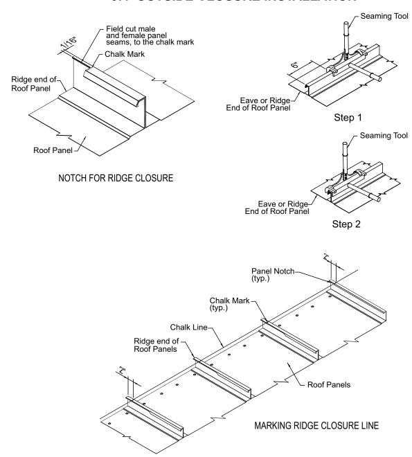
The outside closures should be installed before four roof panel runs are completed. Installation of the outside closures helps maintain the correct roof panel coverage at the ridge. If the outside closures are installed after the roof panels are in place, roof panel coverage error may prevent proper installation of the outside closures.
