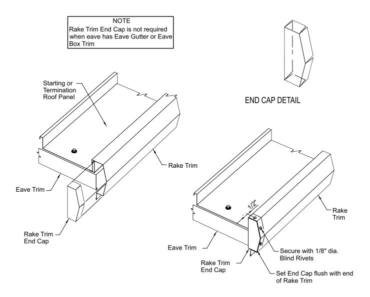
The rake trim end cap is only required for roof applications without eave gutter.
