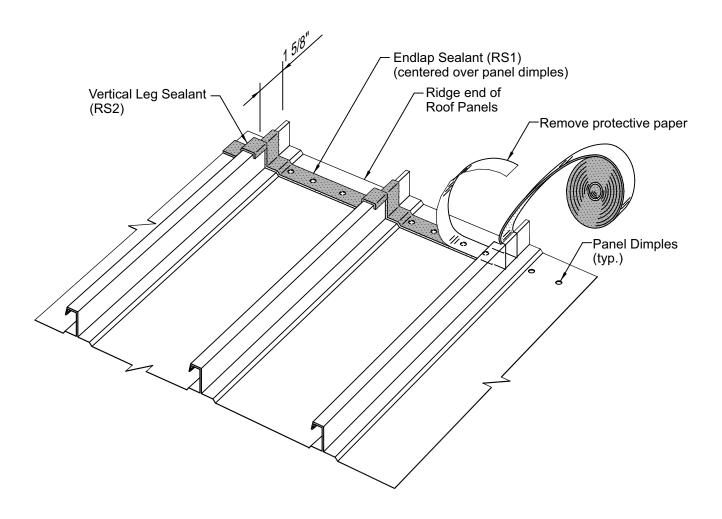
Before installing the endlap sealant, the roof panel's surface must be wiped clean and dry.
