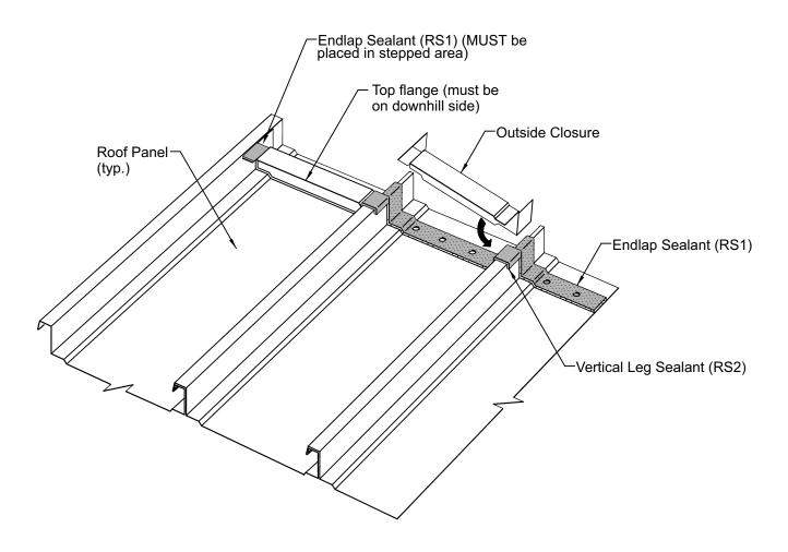
Wipe dry and clean the underside surface of the outside closure flanges.
