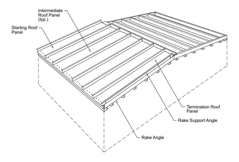
The details in this section show the installation of the termination roof panel.
