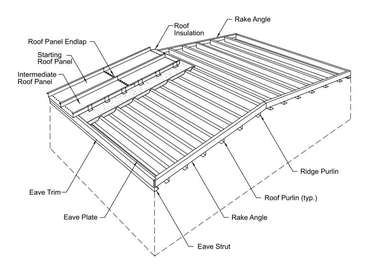
The details in this section show the installation of the starting and intermediate roof panels.
