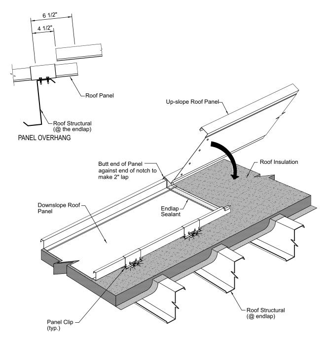
Wipe dry and clean the underside surface of the up-slope roof panel.
