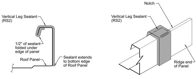
RIDGE PIGTAIL SEALANT DETAIL
