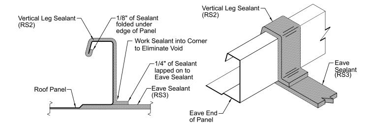
Using a box knife or scissors, cut the sealants to be fitted around the roof panel's seam as shown.
