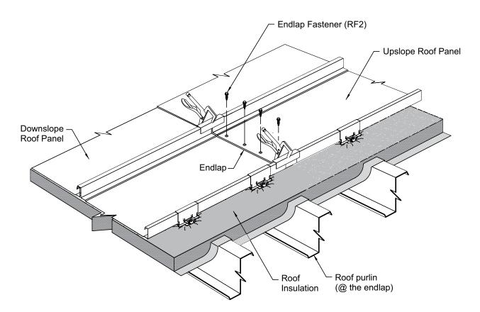
Install roof fasteners in the dimples at each end. Then install fasteners in the remaining dimples.
