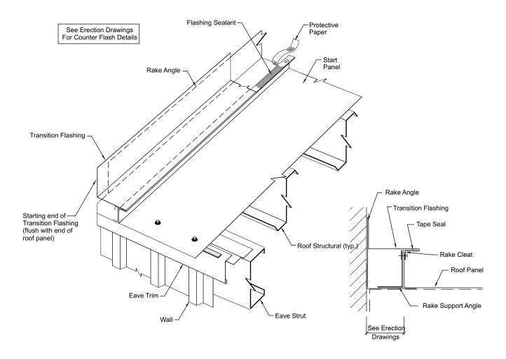
Install the transition flashing from eave to ridge to provide for watershed at the splices
