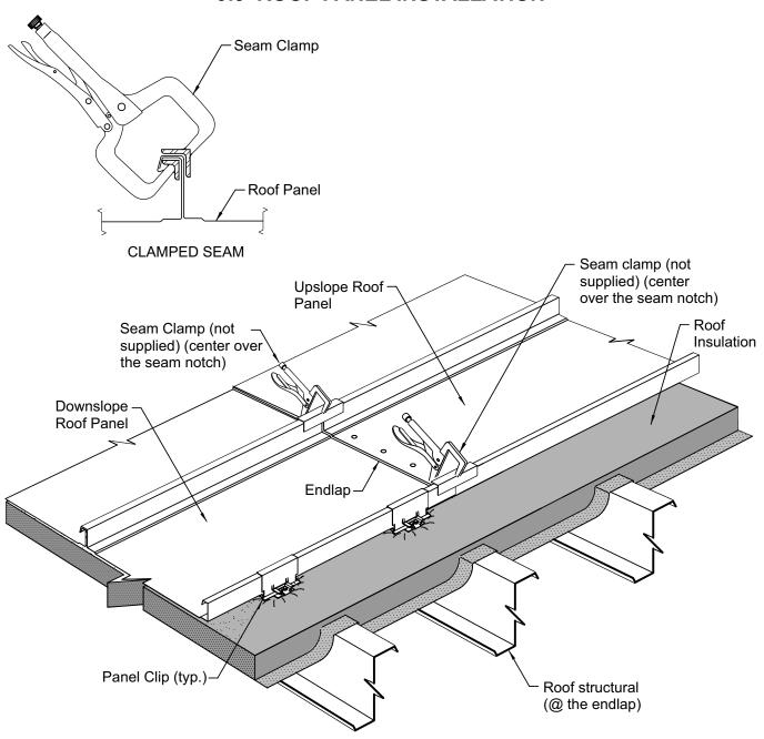
Use the seam clamps to draw the lapping panel seams together as shown.
