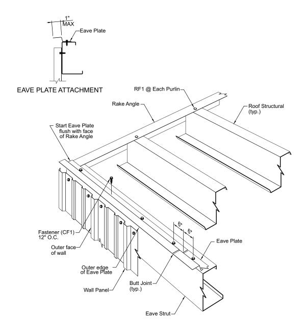
The eave plate may or may not be required when the first purlin space is greater than 4'-0". See erection drawings to determine if eave plate is required. tural members are in straight alignment from rake to rake. Shim the eave plate as necessary to provide a level roof line.
