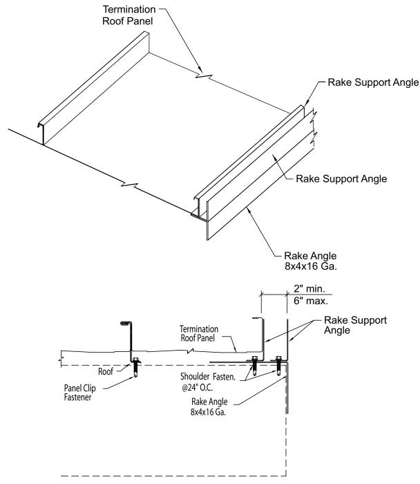
If termination roof panel ends off module at finishing rake, attach additional rake support angle at panel end.
