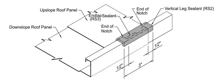
Using a box knife or scissors, cut the sealant to a 3" length and fit around the roof panel's seam as shown.
