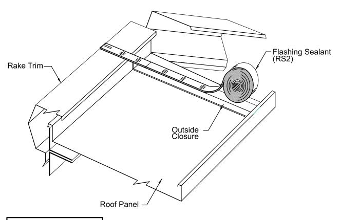
Note: Opposite slope roof panels omitted for clarity.
