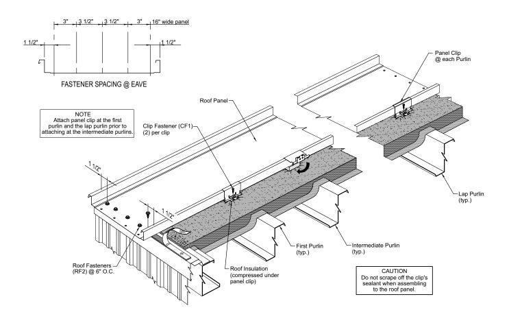
Before fastening the roof panel to the eave plate and fastening the leading edge of the panel with the panel clips, check that the panel coverage is correct and the leading edge of the panel is straight and parallel to the rake line.
