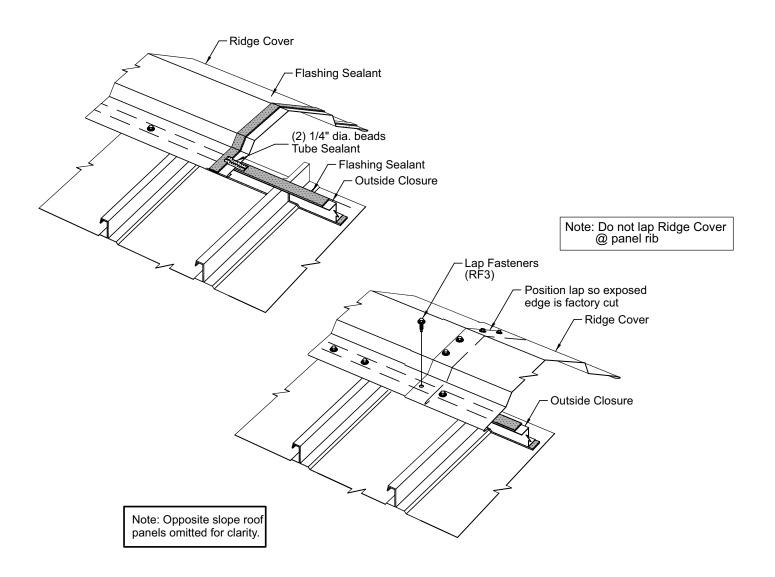
Assemble the ridge cover splices with flashing sealant and lap fasteners as shown.
