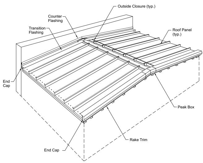
Note: Parapets or existing buildings should extend 1-0" minimum above roof panels.
