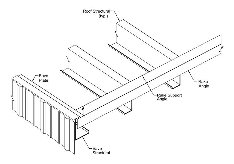
It is important that the rake support angle is installed in a straight line and parallel to the rake line.
