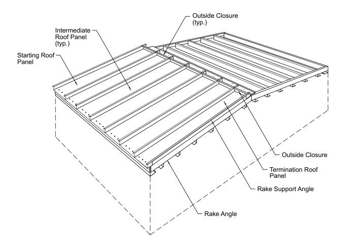
Metal outside closures are used to close the ends of the roofpanels at the ridge, high eave and high eave transition conditions.
