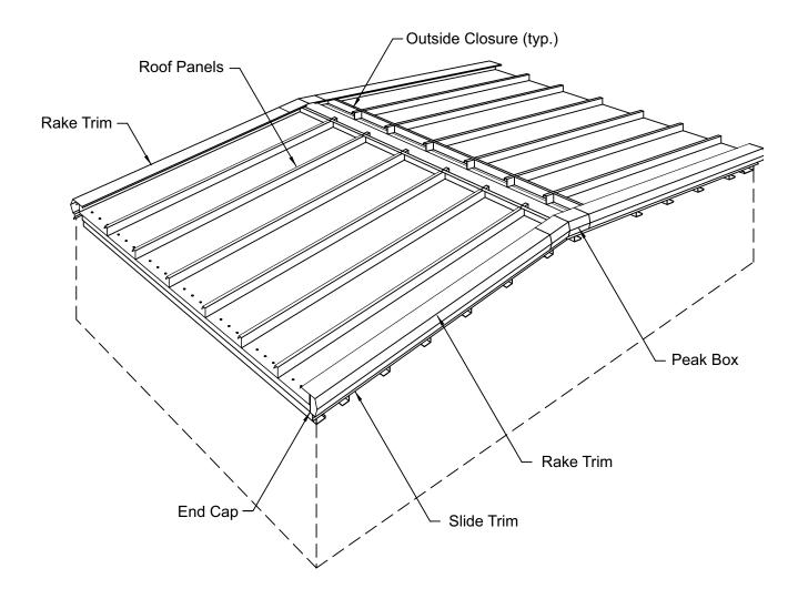
The details in this section show the installation of the rake trim, peak box and end caps.
