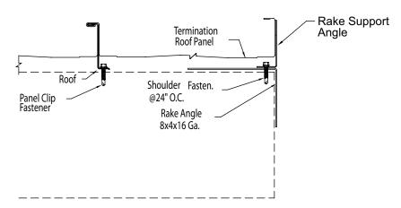
If termination roof panel ends on module at finishing rake, male seam of panel should be against rake support angle.
