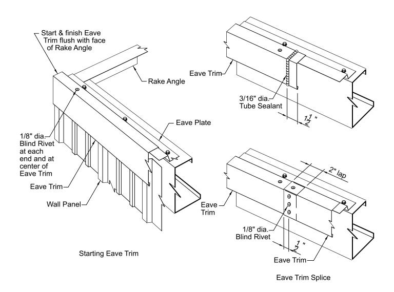
Place the upper lip of the eave trim over the eave plate as shown and align the face of the eave trim with the face of the wall panel.
