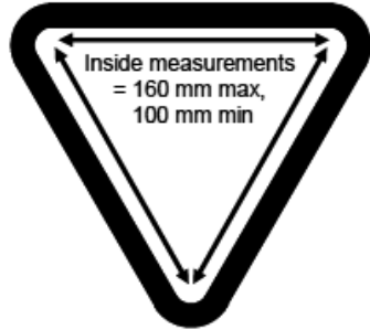
Handle without internal brace (all sides must be equal)
