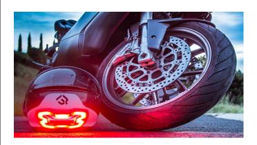
**Brake Free** utilizes accelerometer and gyroscope sensors to *autonomously* detect when you're slowing down no matter how: braking, engine braking, or downshifting. When it does detect you braking, **its LEDs glow brighter letting drivers around you know instantly.** And there is no wired installation or connected apps with your phone for it to work.
