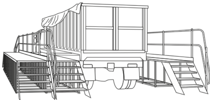
Figure 23. Vehicle sheeting platform
