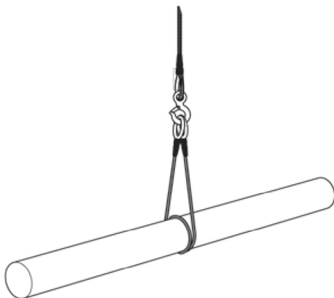
Figure 84. Single sling lift by wrapped choke hitch
