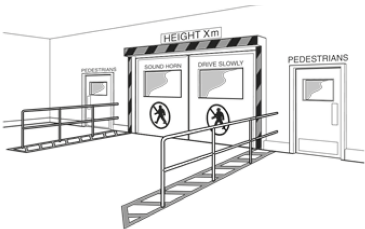
Figure 4. Low doorway markings with maximum heights
