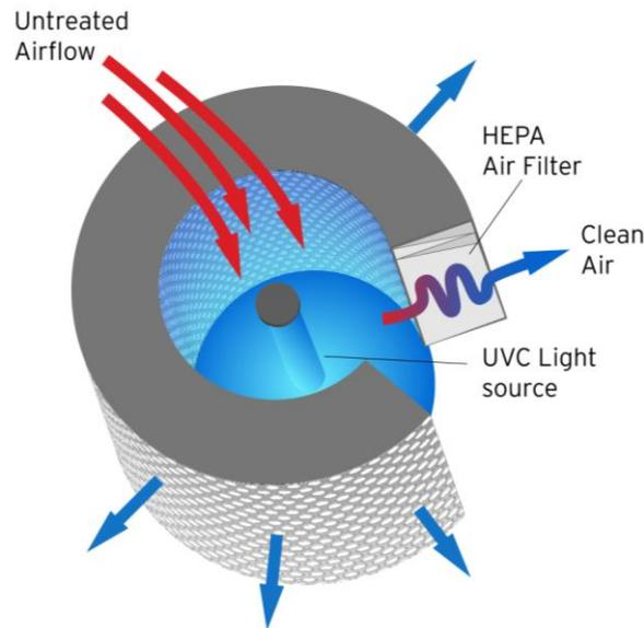
*Figure 10 This "Killer Filter" combines germicidal UV-C with a HEPA filter to kill viruses, fungi and bacteria. Then the inactivated particles are filtered out of the air by the HEPA filter.*
