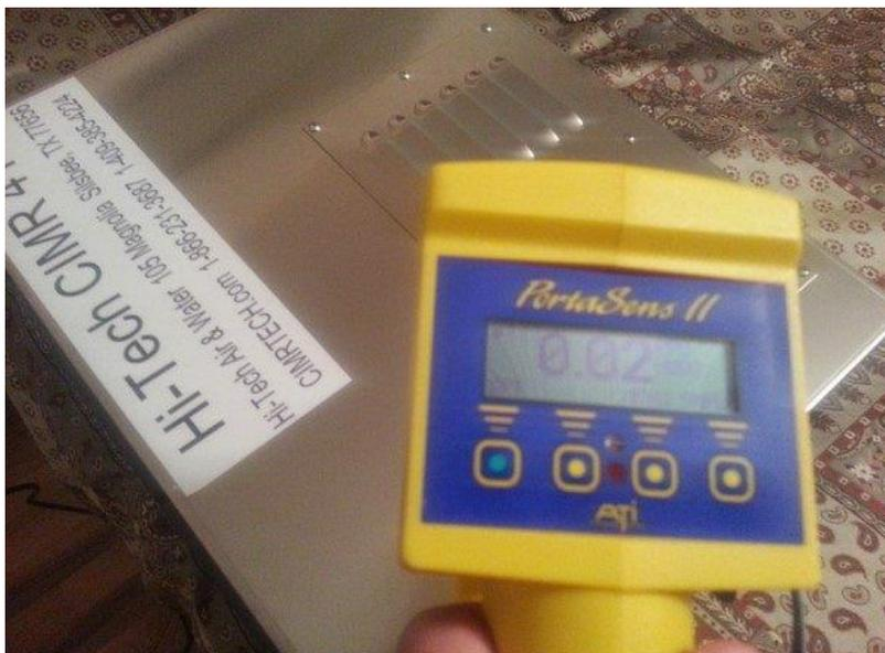
Figure 12 The CIMR 414 from CIMR Technology being measured for hydrogen peroxide in the room. The reading is 0.02 parts per million.
