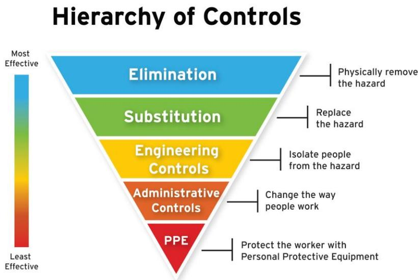
Figure 4 Hierarchy of Controls is used to help assess risks in the workplace.<sup>23</sup>
