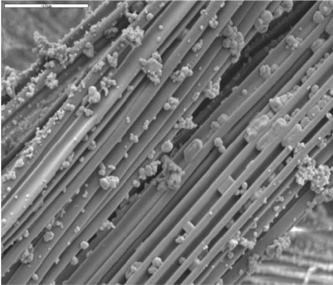
*Figure 9 Scanning Electron Microscope image of Winged Fibers loaded with particles* <sup>32</sup>
