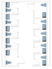
Figure 16 Bathroom design with individual washrooms to limit exposure to a single area.
