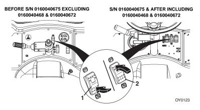
Park brake switch controls the application and release of the park brake. Indicator light on switch illuminates to indicate brake is applied.
