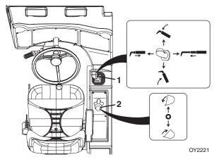
The boom joystick (1) controls lift/lower and extend/retract movement of the boom.
