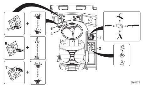
The boom joystick (1) controls lift/lower and extend/retract movement of the boom. The attachment tilt joystick (2) controls fork tilt.
