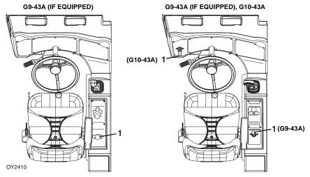
• Auxiliary hydraulic joystick (1) controls function of attachments that require hydraulic supply for operation. See Section 5 - Attachments for approved attachments and control instructions.
