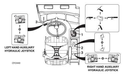
The boom joystick (1) controls lift/lower and extend/retract movement of the boom.
