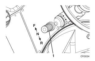
Transmission control lever (1) engages forward or reverse travel.
