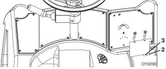
The lubrication and maintenance decal (1) or lubrication (2) and maintenance (3) charts contain instructions that must be followed to keep this product in good operating condition. The Operation & Safety Manual and Service Manual contain more detailed service information with specific instructions.
