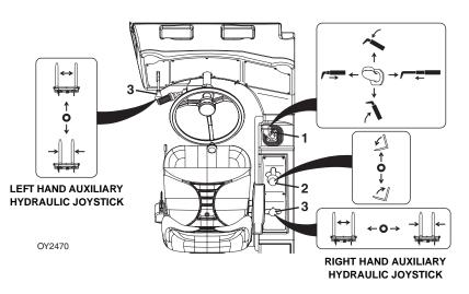
The boom joystick (1) controls lift/lower and extend/retract movement of the boom.
