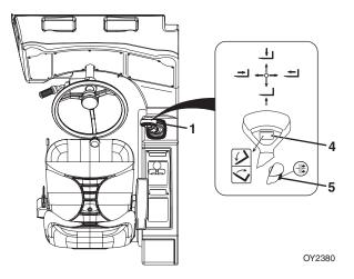
The boom joystick (1) controls the boom, attachment tilt and clutch lock functions.
