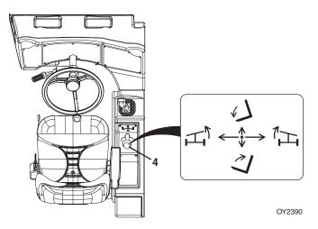
The middle joystick (4) controls the left to right frame level and attachment tilt (if equipped) functions.
