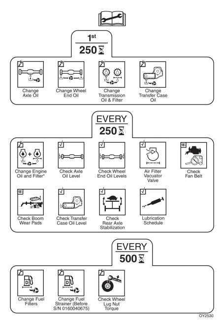
**Note:** Engine oil and filter service interval can be extended, see page 7-14 for details.
