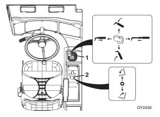
The boom joystick (1) controls lift/lower and extend/retract movement of the boom. The attachment tilt joystick (2) controls fork tilt.
