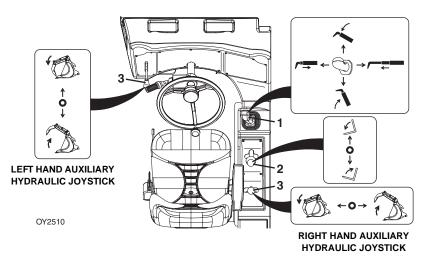
The boom joystick (1) controls lift/lower and extend/retract movement of the boom.
