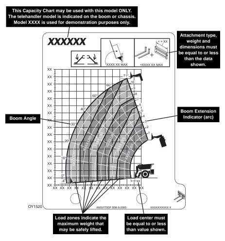
**Note:** This is a sample capacity chart **only**! **DO NOT** use this chart, use the one located in your operator cab.
