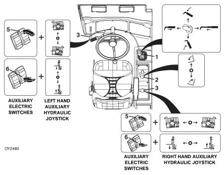
The boom joystick (1) controls lift/lower and extend/retract movement of the boom.
