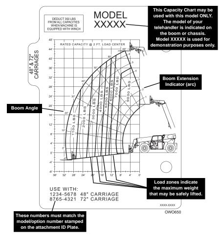
**Note:** This is a sample capacity chart **only**! **DO NOT** use this chart, use the one located in your operator cab.
