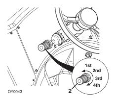
Gear selection is located on the twist grip handle (2) of transmission control lever.
