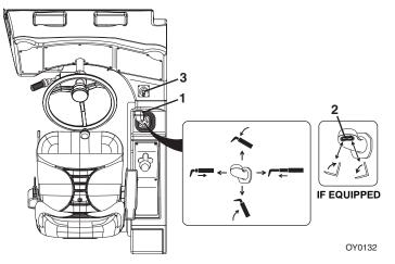
The boom joystick (1) controls the boom and attachment tilt (if equipped) functions.
