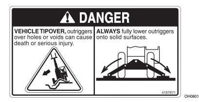
Lowering outriggers over holes or on soft terrain can compromise the stability of the vehicle which could result in vehicle tipover. For optimum stability, lower the outriggers just far enough until the front of the vehicle starts to raise and maintains a <u>firm</u> footing.
