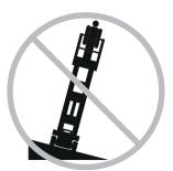
Do not depend on the tilt alarm as a level indicator. The tilt alarm sounds only when the machine is on a slope.
