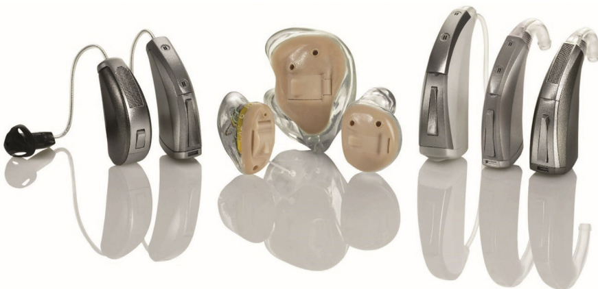
Fig. 5. Modern hearing aids. These hearing aids can stream acoustic signals from electronic devices, such as cell phones and tablets, directly to the hearing aids. (Courtesy of Starkey Laboratories, Eden Prairie, MN; with permission.)
