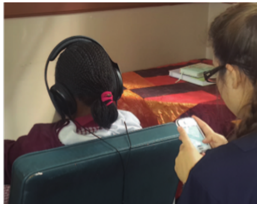
Figure 5. Clinical hearing screening test on school child using smartphone with hearScreen™ application and HD202 headphones. Phone is held upside-down to ensure the microphone faces towards the test subject for environmental noise monitoring.
