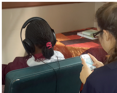
Figure 5. Clinical hearing screening test on school child using smartphone with hearScreen™ application and HD202 headphones. Phone is held upside-down to ensure the microphone faces towards the test subject for environmental noise monitoring.
