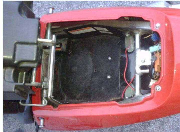
9) Insert undertail left side first, then right side, be carefully not to crack or scratch undertail. Tighten light first, then all other bodywork mounting locations, then insert 2 screw rivets into stock locations into undertail.
