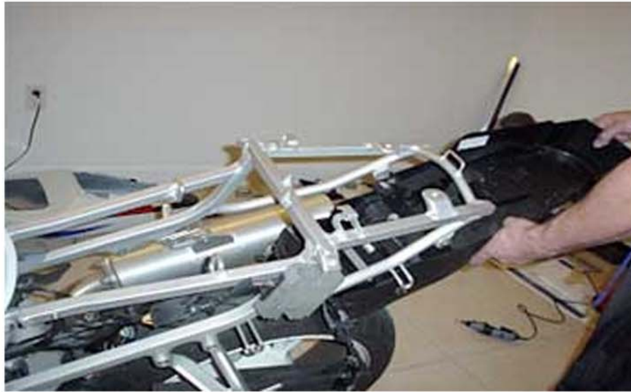
(Inner Fender Being Removed)
