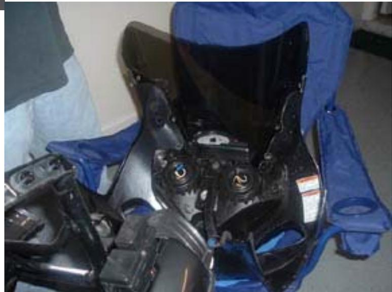
**3-Remove 4 screws holding headlight & speedometer.**
