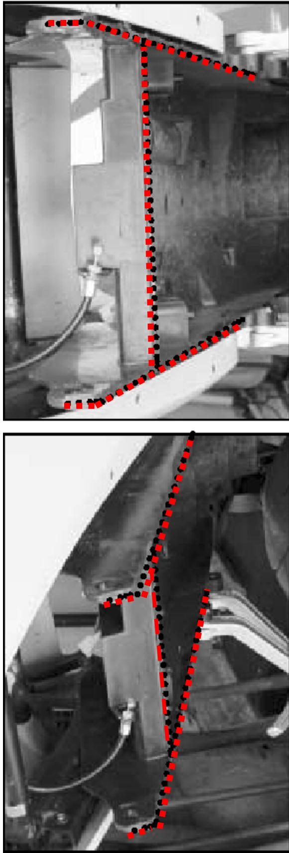
4-Using a Dremel or hand saw, remove the plastic shown in the pictures.
