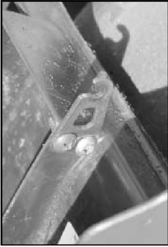
5-Drill 2 holes (using a 10/32" bit) for the installation of the lock cable mounting arm.
