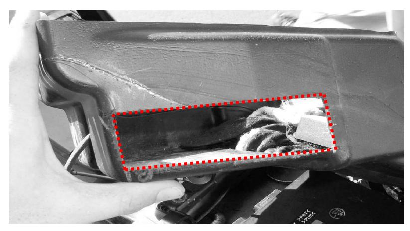
Cut Inner glove box to allow ECU to fit inside.
