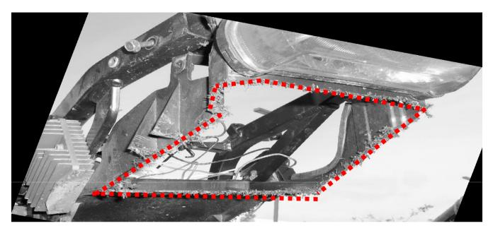
Carefully remove the tail section body work.
