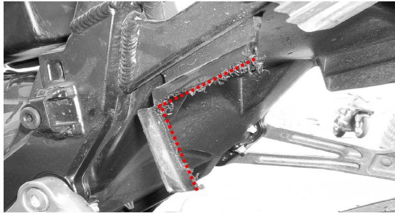
Using a "Dremel" tool or hand saw, remove the plastic shown in the next pictures. Be sure to take your time cutting, so that you don't cut away any more plastic than necessary.
