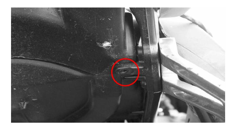
Remove bolts attaching the subframe to the battery box near the passenger foot pegs
