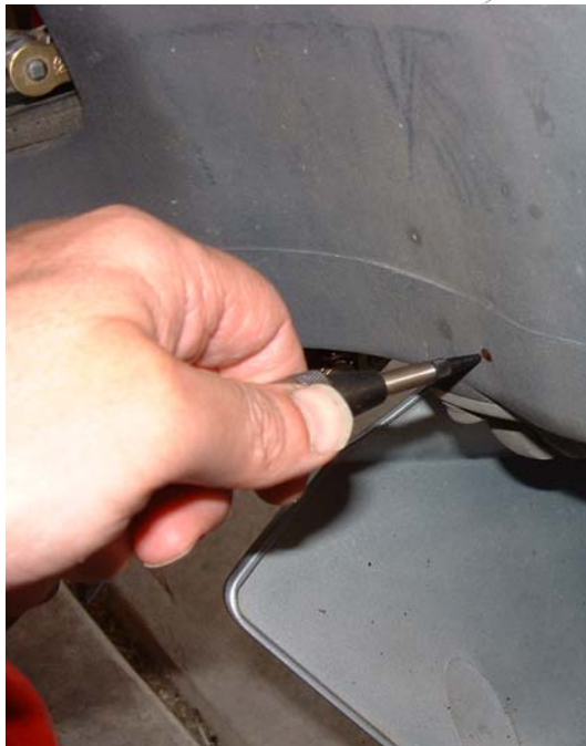
1. Center punch in the middle of each dot
