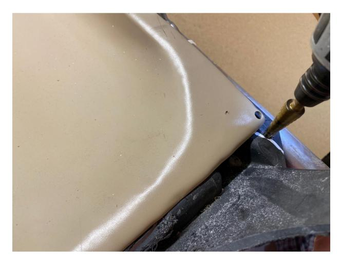
Align the undertail with the tray. Once everything is aligned (top and bottom) proceed to drill 1 hole on each corner
