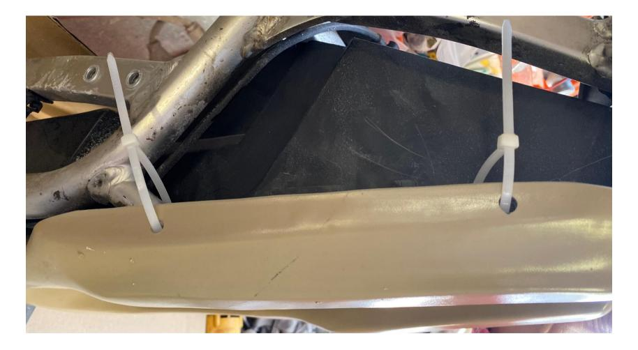
Once everything is completely in place and aligned, install the tail section and FASTEN all 4 zip ties (top & bottom).
