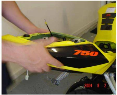
Place back the tail section. Leave it loose. Do not bolt it in yet until after you install the undertail (for easy handling)
