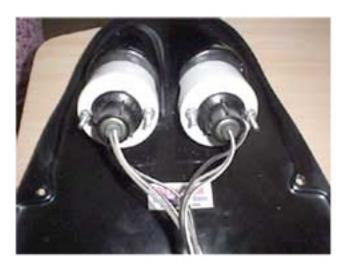
NOTE: It's easier for you to assembly the tail lights before installing the undertail.
