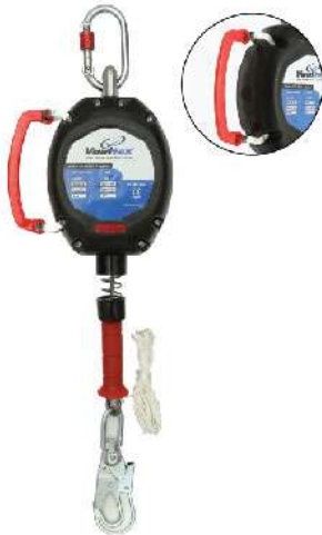
STYLE NO: ICV BRAND: VAULTEX RETRACTABLE FALL ARRESTER - 7.5 METER 4.8 MM STEEL ROPE | CAPACITY: 100 KG EN 360:2002 / ORIGIN: INDIA
