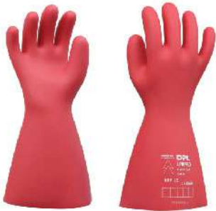
STYLE NO: THU BRAND: LINEPRO LATEX ELECTRICAL GLOVES 36CM CLASS 1 (7,500V AC) EN 60903:2003/IEC 60903:2014 CAT III TYPE 1/CE 0598 SIZE: 9 / ORIGIN: SRI LANKA
