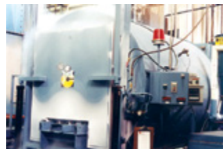
CRYOGENIC TREATMENT Temperatures to -300°F
