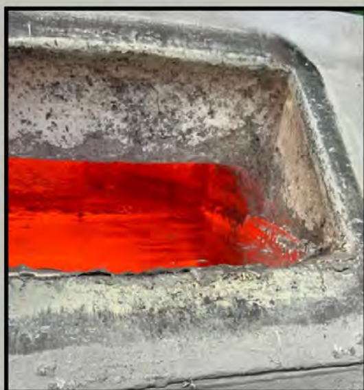
WAM® AL II AFTER 28 MONTHS OF OPERATION
