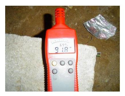
Vented crawl spaces can also get cooler than 80° F. I took the photo of the hygrometer above on a warm August day here in the Atlanta area, and you can see that the air was about 70° F with 92% RH.
