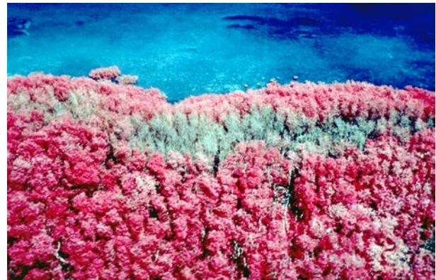
Figure 3.2. Infrared aerial photograph of a band of dead mangroves where oiling was heaviest on the prop roots and penetrated into the soils. Note the lighter color of the outer fringe mangroves indicating stress. This is a classic example of inner fringe impact (Research Planning, Inc.).
