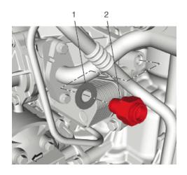
**Note:** The turbocharger coolant feed pipe fitting is not reusable.
