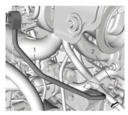
4. Clip in the turbocharger coolant feed pipe (1) to the turbocharger coolant feed pipe fitting (2).
