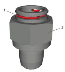
1. The clamp (1) from the turbocharger coolant feed pipe fitting (2) is pre installed.
