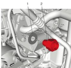
2. Install a NEW turbocharger coolant feed pipe fitting gasket(1).
