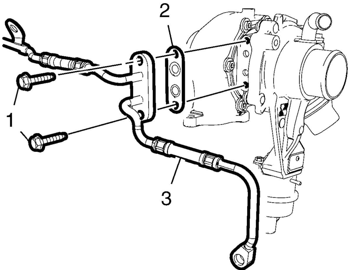
2. Remove the 2 turbocharger coolant feed and return pipe assembly bolts (1).
