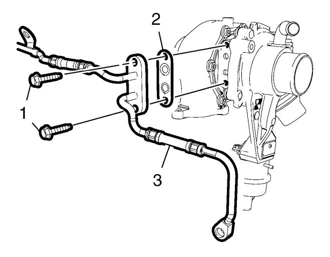
1. Install the turbocharger coolant feed and return pipe assembly (3) and a NEW gasket (2).
