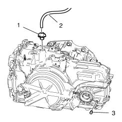
**Warning:**The engine must be running when the transmission fluid fill plug is removed, or excessive fluid loss will occur. Transmission fluid may be hot. Since the actual fluid level is unknown, stand clear when removing the fill plug. Have a container ready to capture any lost fluid. Do not turn the engine off with the fill plug removed, as you can be injured by hot transmission fluid being expelled out of the oil fill opening.
