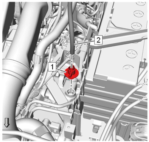
8. Remove the transmission vent hose (2) and the transmission fluid filler cap (1).
