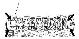
**Note:**Ensure that the cylinder head surface (1) is clear of oil, grease and old gasket material.
