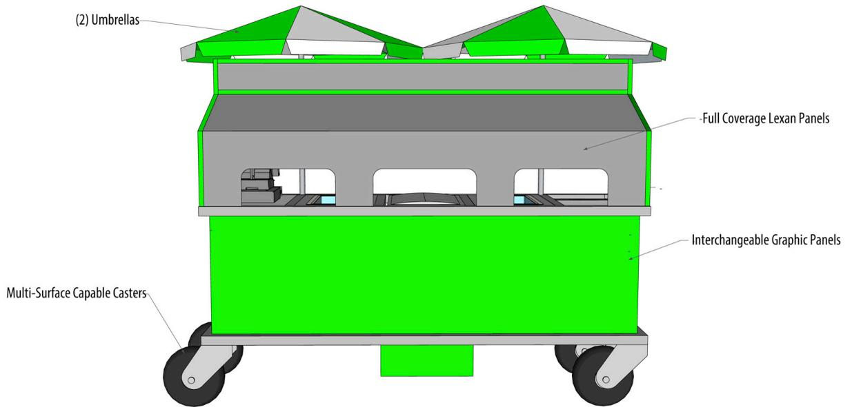
**The OFF-ROAD FOOD CART** is designed for transporting across virtually any surface. The pneumatic casters are designed to travel over rough surfaces such as dirt, grass, cracked concrete and asphalt.
