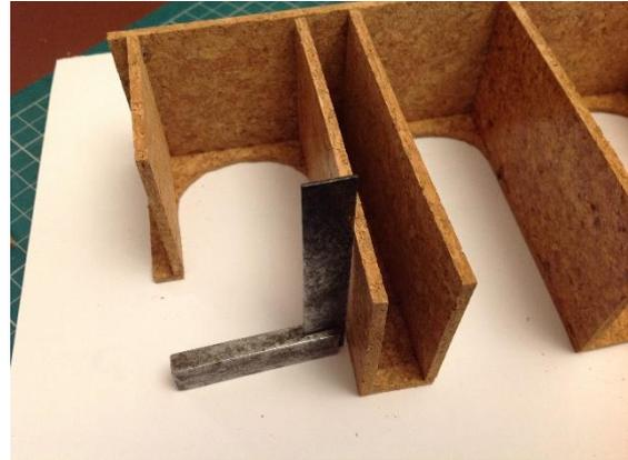
3 Glue on the other bridge side and use pins or small pieces of masking tape to hold everything square until the glue sets. Then tidy up all cut edges.
