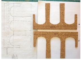
2 Draw and cut out the transverse leg faces and the trackbed. Lay one bridge side down and glue the trackbed and transverse leg faces. An engineer's square or similar is a necessity at this stage.
