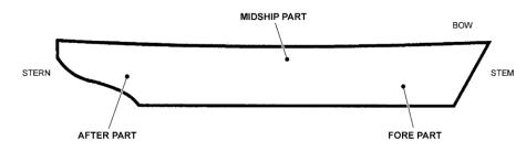
After Part. The part of the hull ending at the stern.
