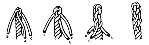
CLOSING STATEMENT - A back splice is a useful and effective means of finishing the end of a line.
