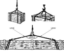
When using strops for hoisting, the angle between the legs of the sling will determine the amount of stress the strops must endure. The recommended angle of work is between 0 degrees and 120 degrees.
