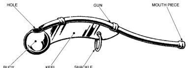
BUÓY KEEL SHACKLE **Gun.** The long portion that runs along the top of the boatswain's call through which air is blown. The mouth of the gun is the ridged portion that is placed in the mouth.
