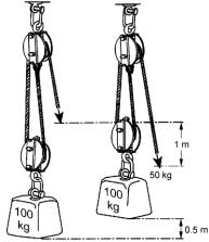
If the distance the load must be moved and the VR are known, calculate the hauling part distance using the following formula:
