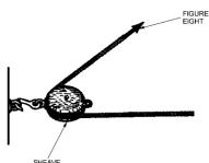
**CLOSING STATEMENT -** For a block to work efficiently the line must move freely; therefore lines should be free of kinks and tangles when reeving blocks. This skill will be applied in future rigging tasks.
