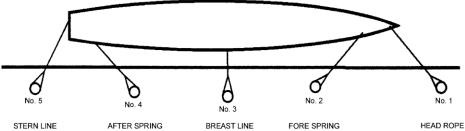
A ship's berthing arrangement depends on the size and characteristics of the ship. Each berthing line has a special name and purpose, which are as follows:
