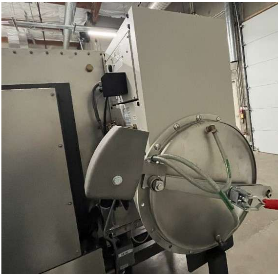
Left glovebox – Rear view of vacuum oven with water cooled doors
