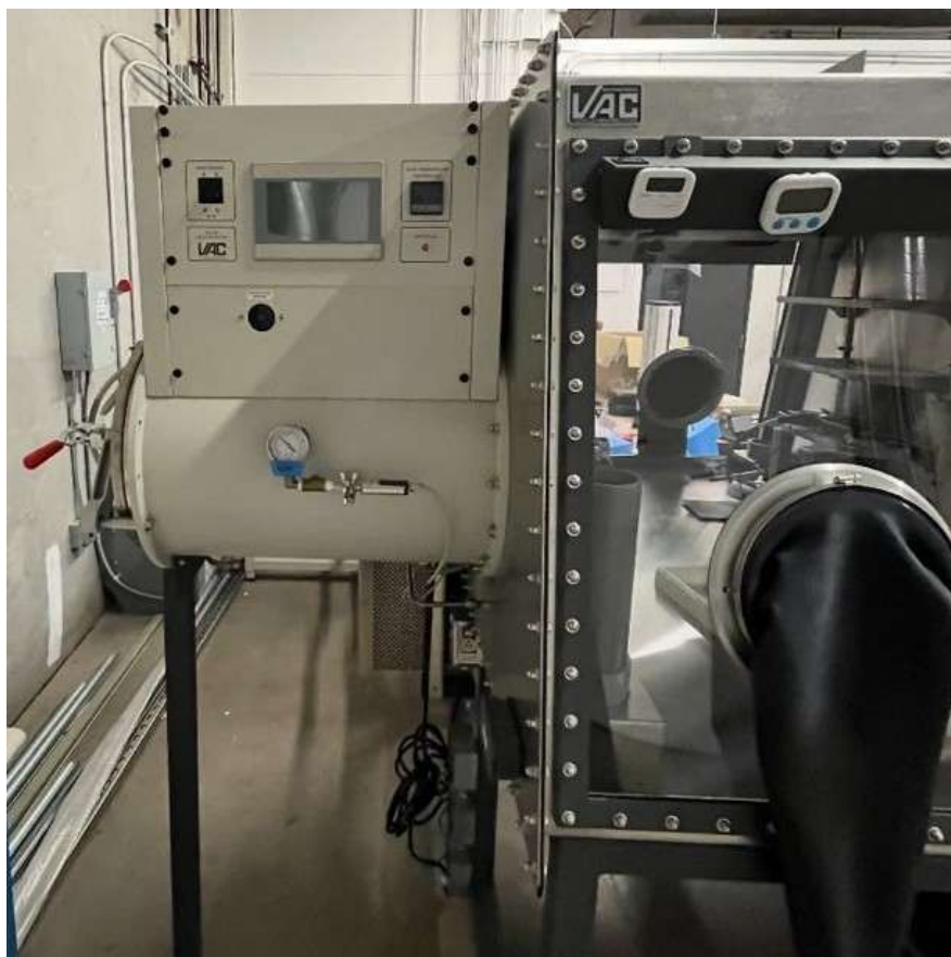
Left Glovebox – Vacuum oven 600 degree C
