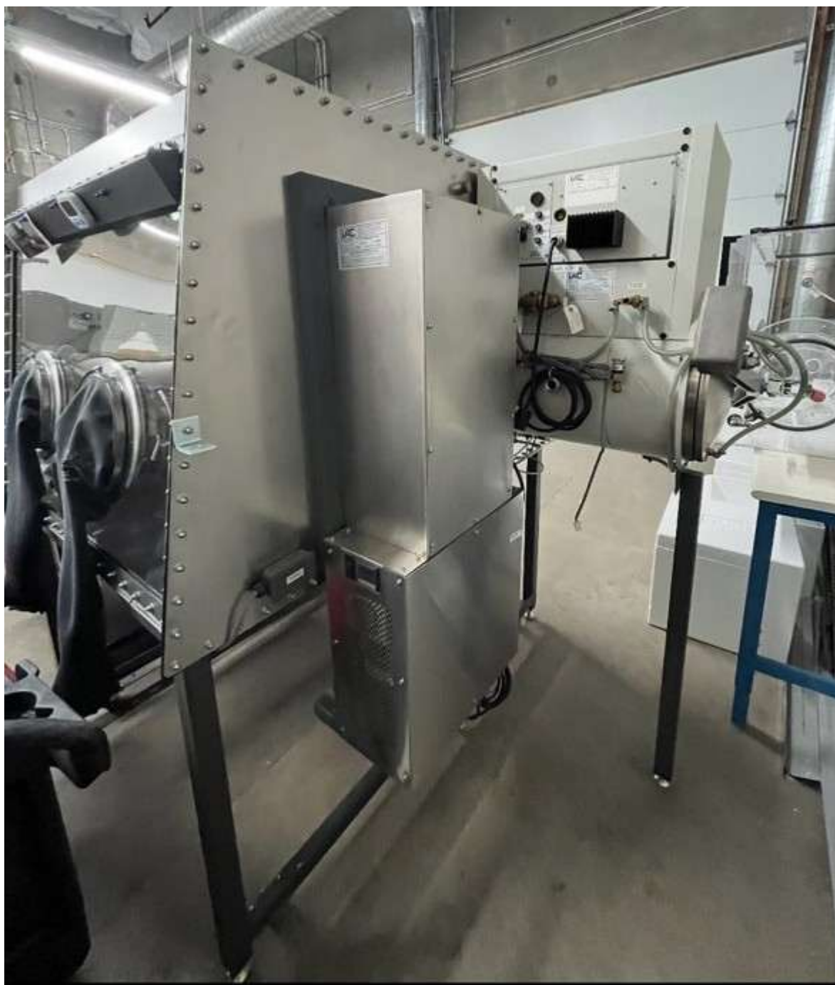
Left glovebox – view of rear window and cold storage unit -40 degree C
