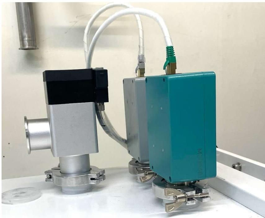
View of the O2 & H2O sensors and the purge valve located on top of the glovebox.
