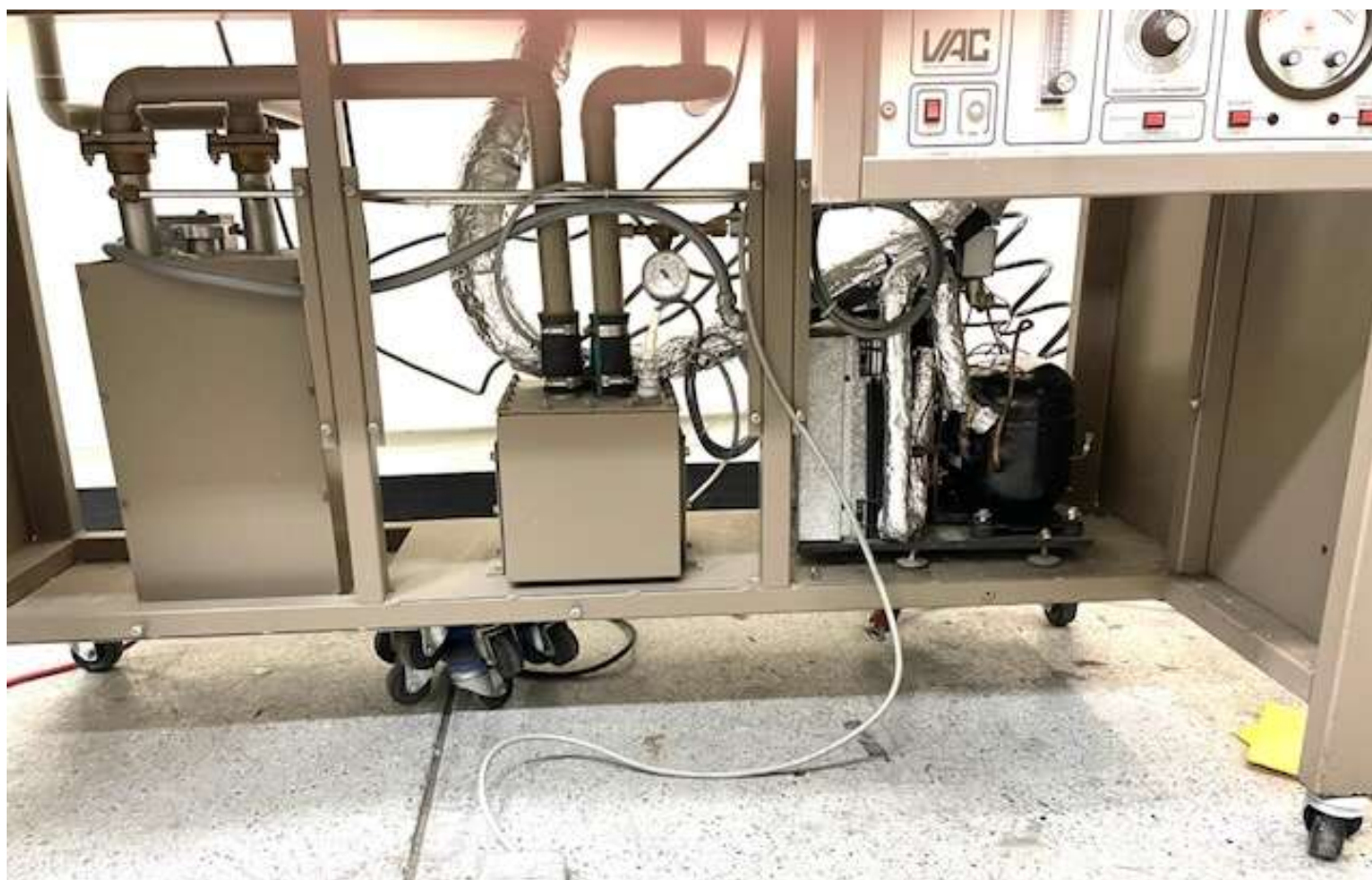
Powerful purifier with large capacity catalyst bed with new catalyst installed
