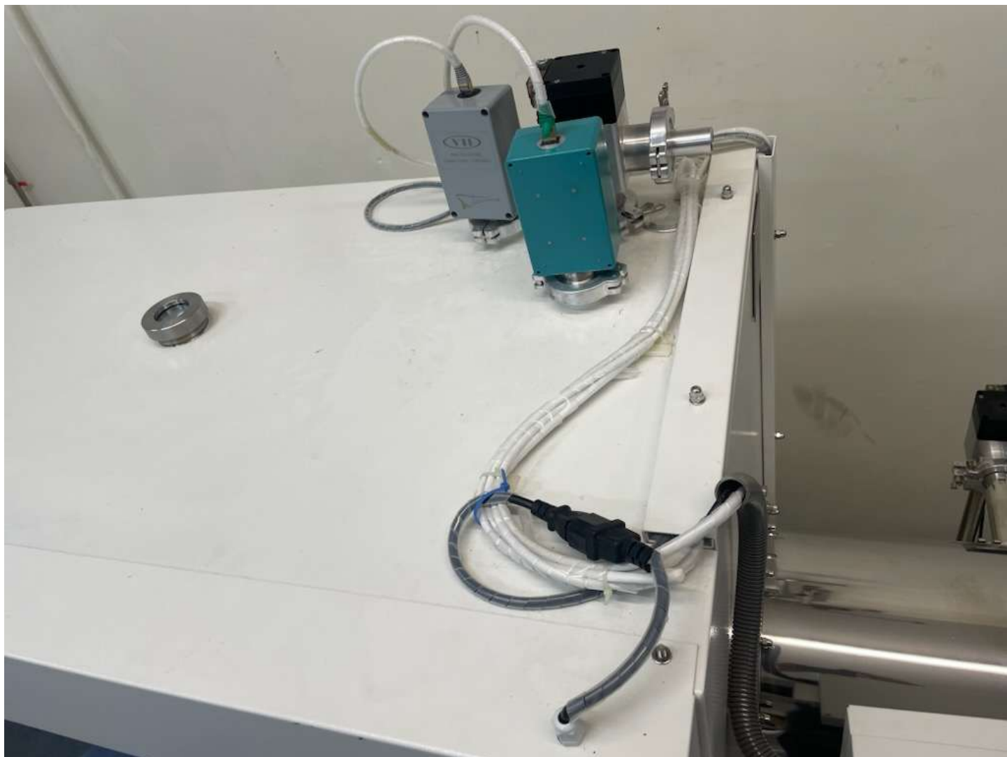
View of the O 2 & H 2 O sensors, purge valve & quartz window located on top of the glovebox.
