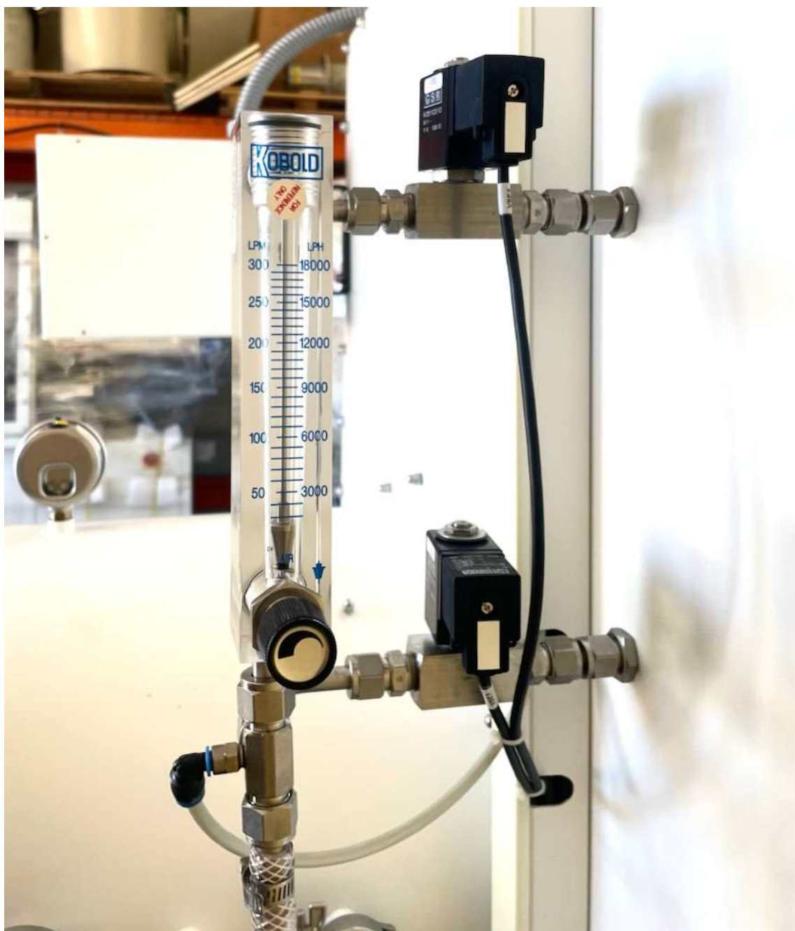
Manual purge flow control valve with indicator and automated flow shut off valves
