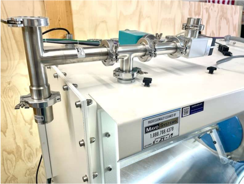
Top mounted purge exhaust plumbing with pneumatic shut off valve and H2O sensor
