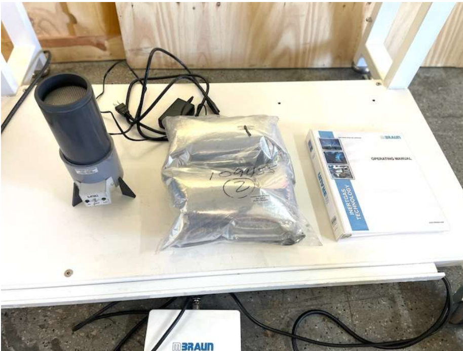
VAC Genesis Purifier with Included pre-regenerated moisture cartridges
