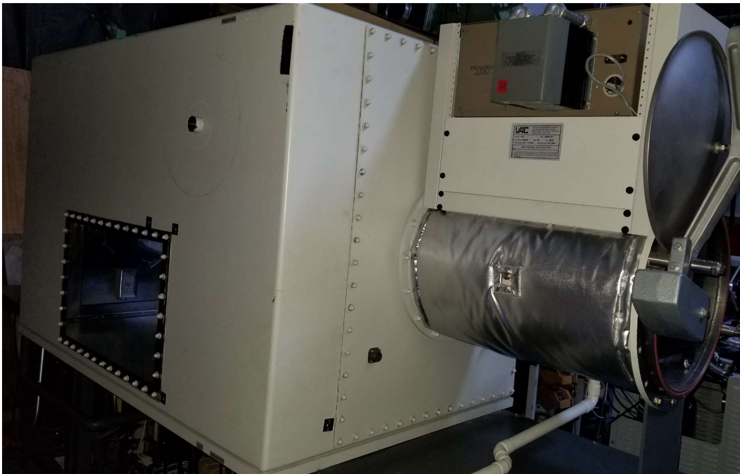
Rear view showing back window. Option of adding a gloveport and KF 40 feed thru
