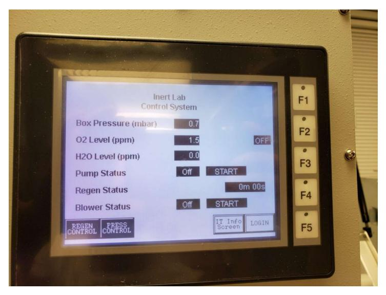
This system is a purge system which requires a constant flow of inert gas to maintain an atmosphere. This system does NOT have a purifier with regen control.
