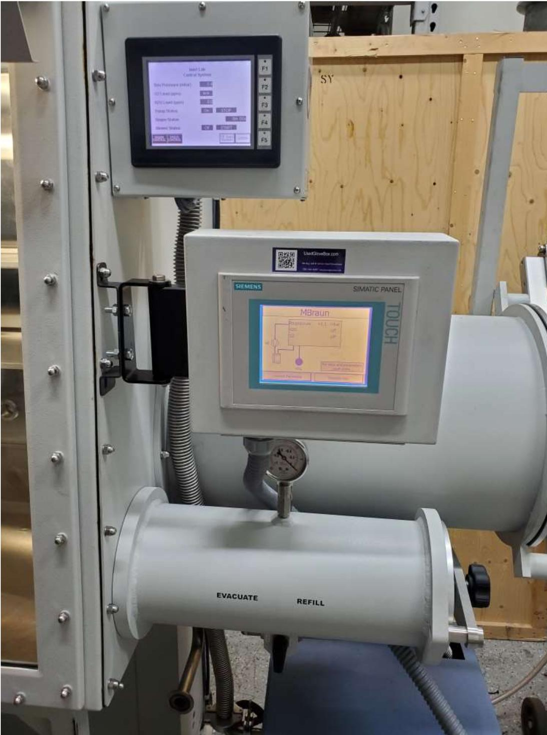
The *Inert* glovebox control (top) is for display of the O<sub>2</sub> level. The *MBraun* purifier touch screen control is for circulation, regeneration, and pressure control.
