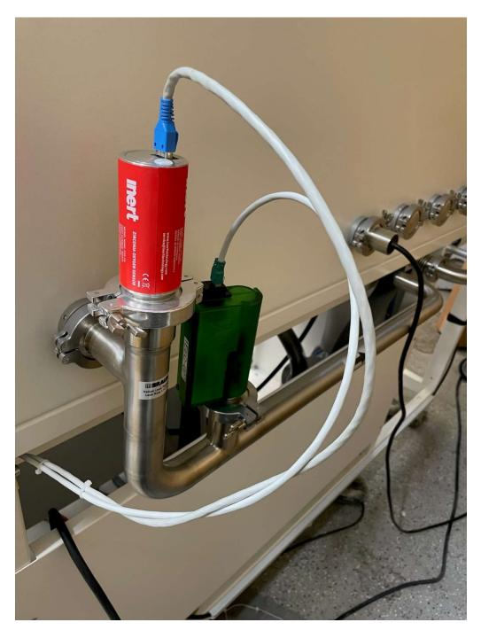
Inert Corp O2 & H2O sensors. The sensors read out on the MBraun control panel. The sensors are refurbished, calibrated and have a one year warranty.
