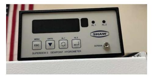
Used *Shaw Superdew 3* Dewpoint Hygrometer operates independently from the glovebox controls read to equivalent of 1 ppm H2O. Includes aluminum oxide probe sensor that reads directly from box atmosphere. Probe calibration is not guaranteed.
