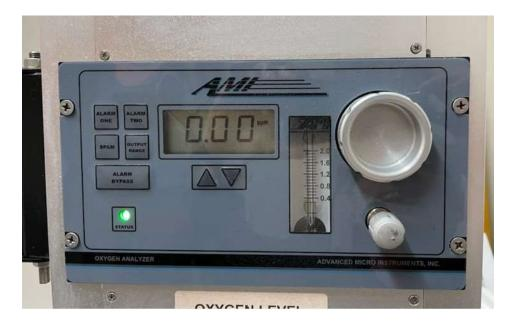
Used *AMI* Oxygen Analyzer integrated with the MBraun system. Sensitivity rating of 1 ppm. Includes sample pump with sample line and return line. The instrument is used calibrated, nothing additional required for calibration. A new KOH fuel cell sensor and operation manual will be provided.
