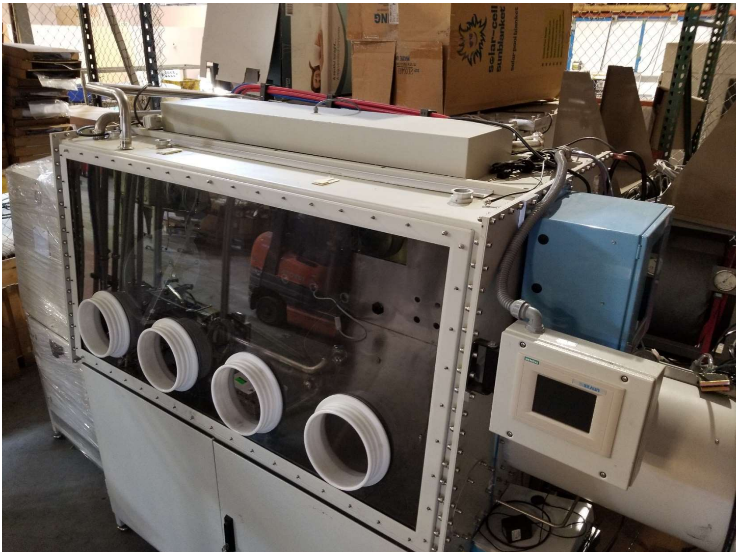
Top view of glovebox showing skylight, the blue box is a gas mixer which is not included
