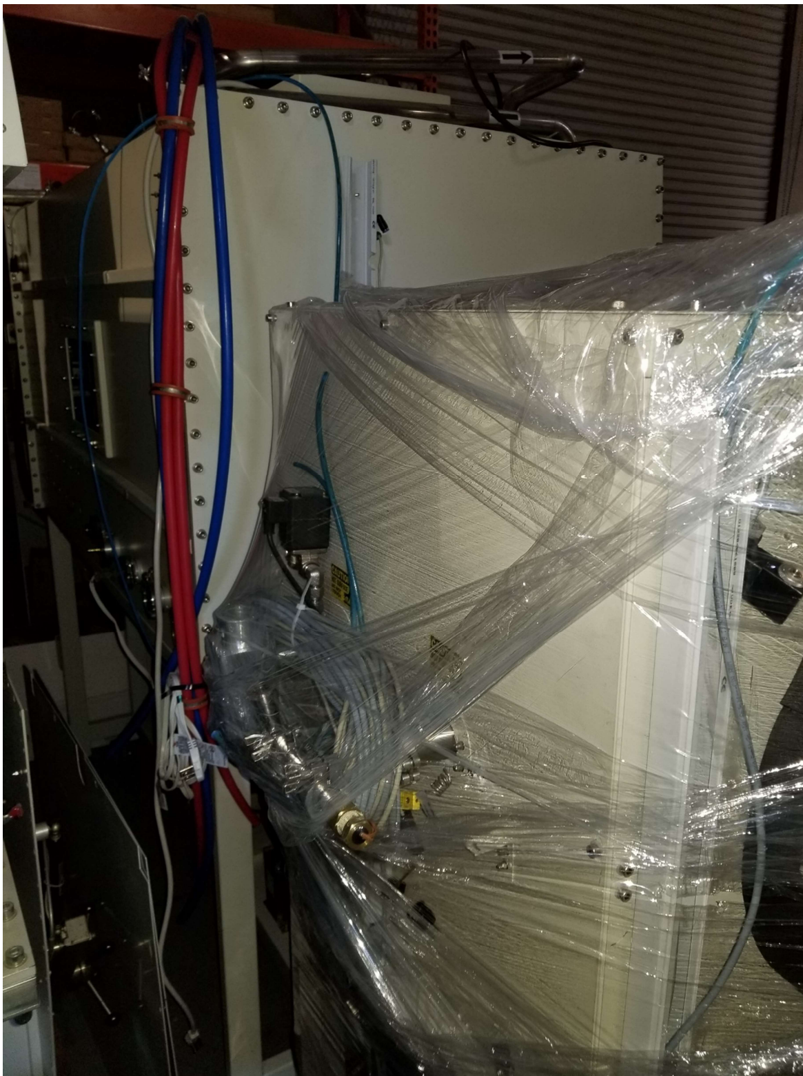
Back view of glovebox and vacuum oven showing evacuation and refill valves
