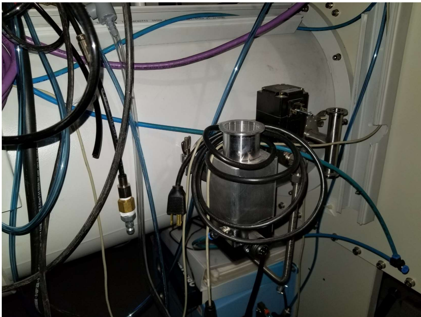
Back view of antechamber showing the evacuation and refill valves
