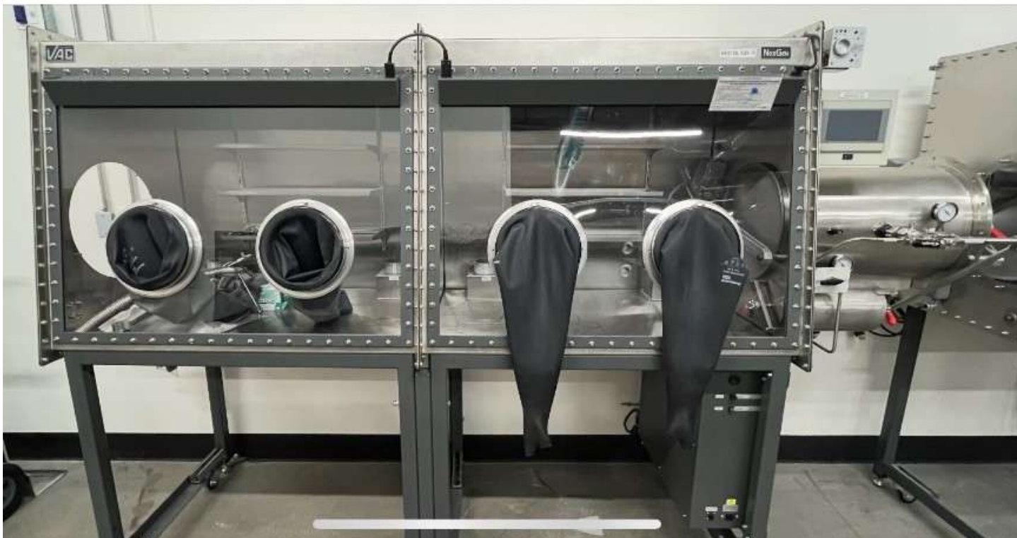
Right glovebox – front view
