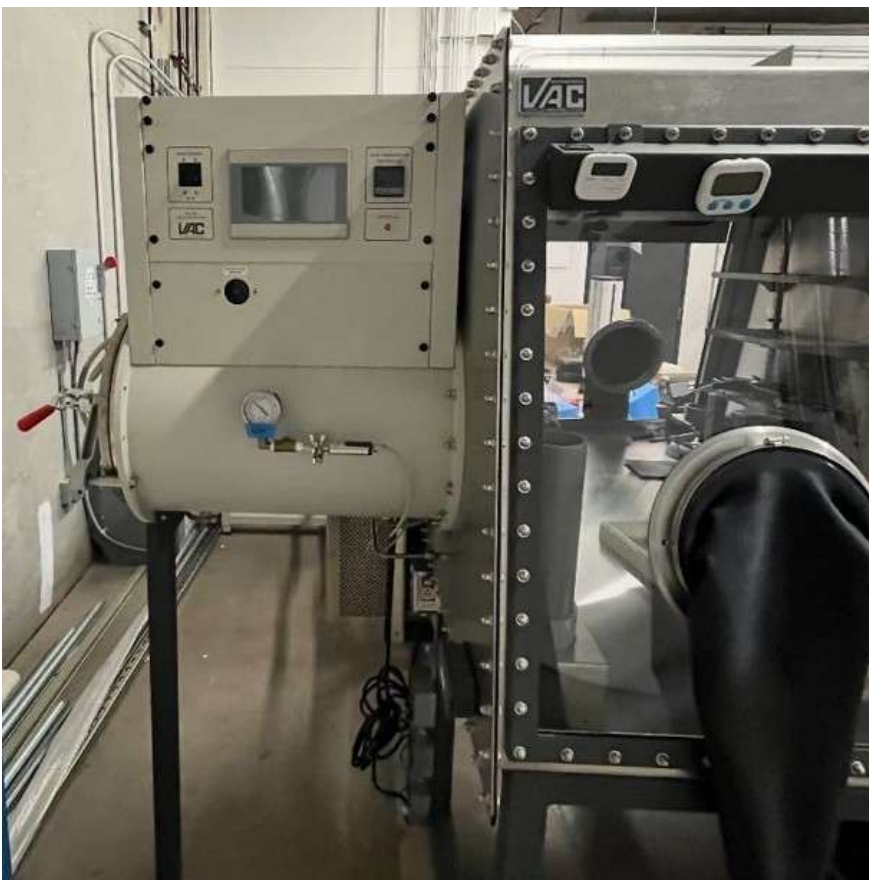
Left Glovebox – Vacuum oven 600 degree C
