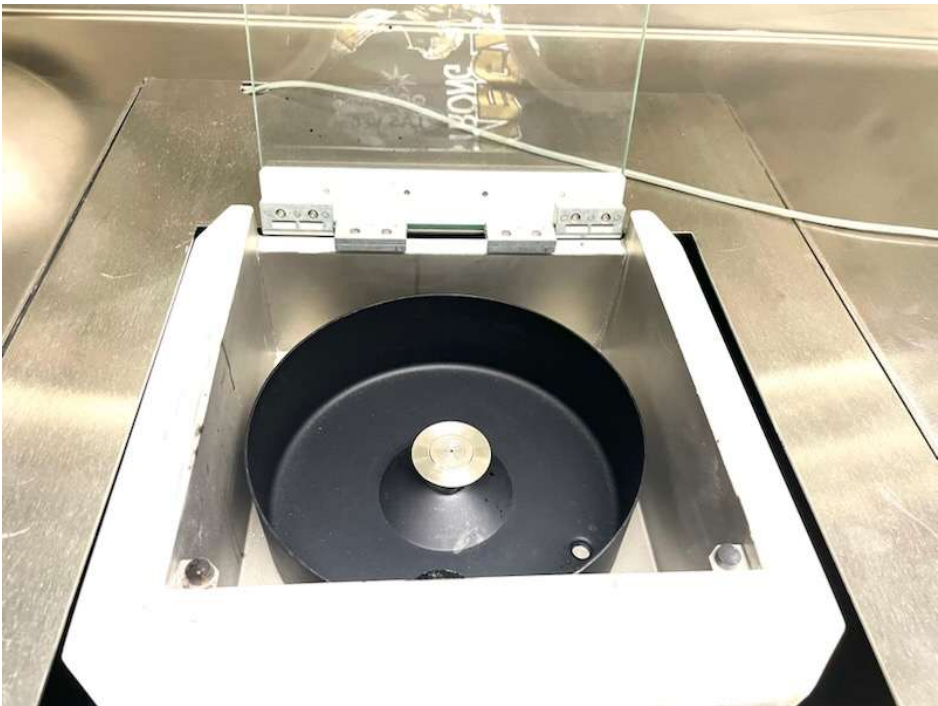
Spin Coater integrated within a well
